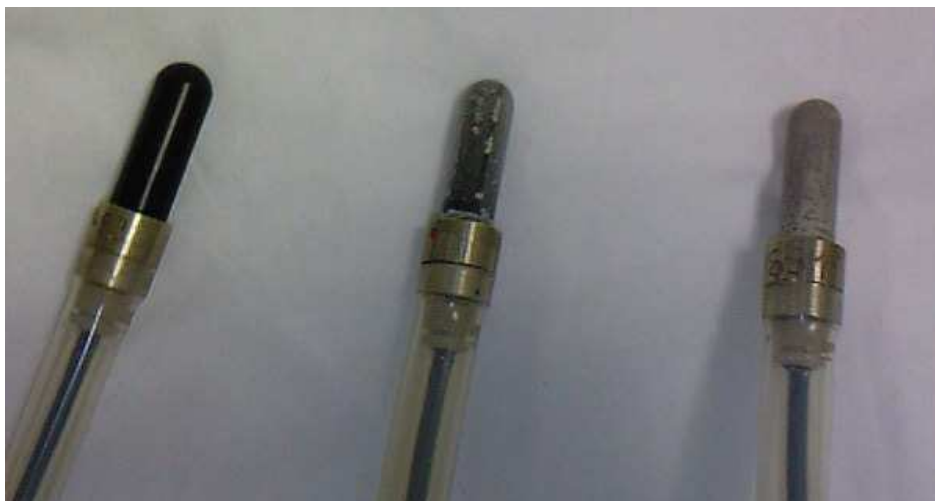
Figure A.1: The three used gas flushed ionisation chambers: TE/TE, MgB/Ar and Mg/Ar chamber. All three chambers are of similar design and dimensions.
