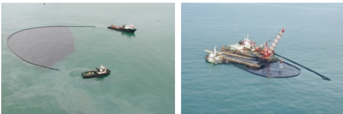
Booms being used to contain and concentrate floating oil
