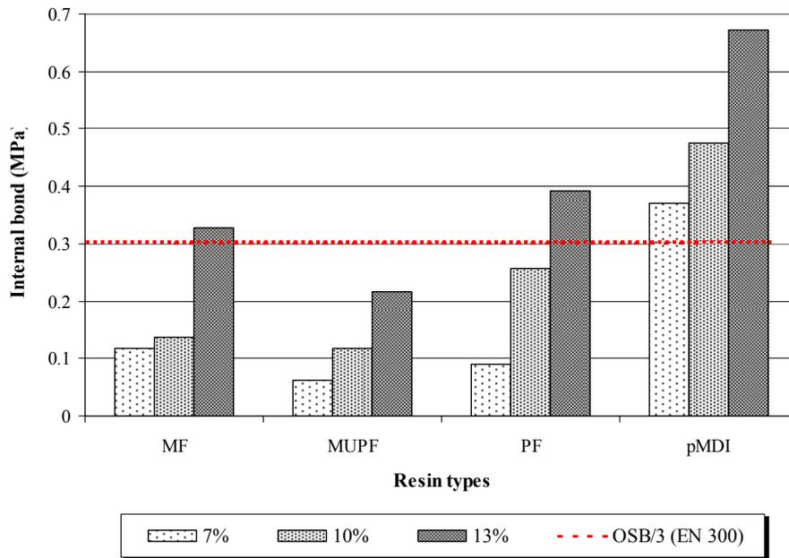
Fig. 6 Internal bond of bamboo-based OSL
