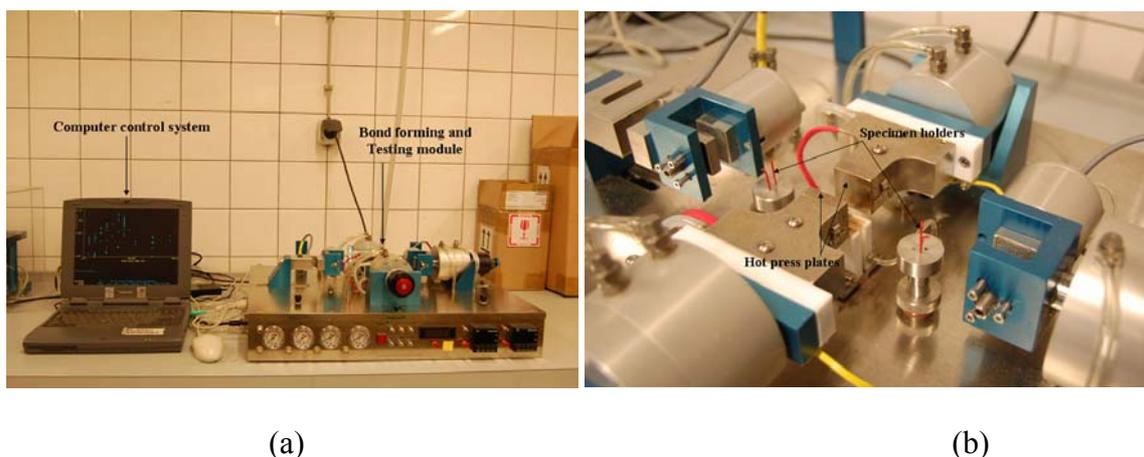
**Figure 1** Features of Automated Bonding Evaluation System device, (a) The ABES system composing of the bond-forming and testing module and computer control system (b) A close-up of the bond pressing zone composed of the hot press plates and specimen holders.
