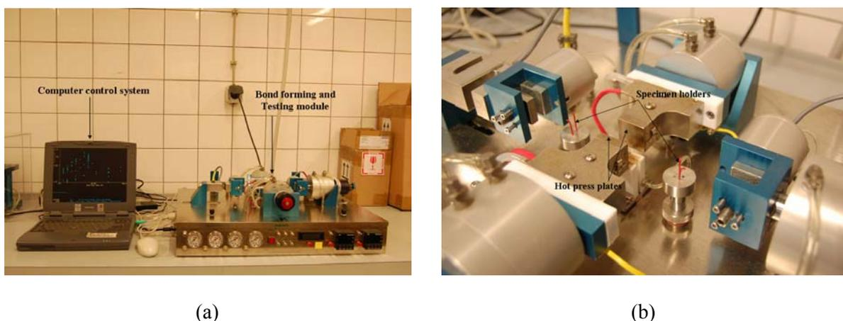
Figure 1 Details of Automated Bonding Evaluation System device, (a) ABES overview, which is composed of the bond-forming with testing module and computer control system (b) A close-up of the bond forming zone, which is composed of the hot press plates and specimen holders.
