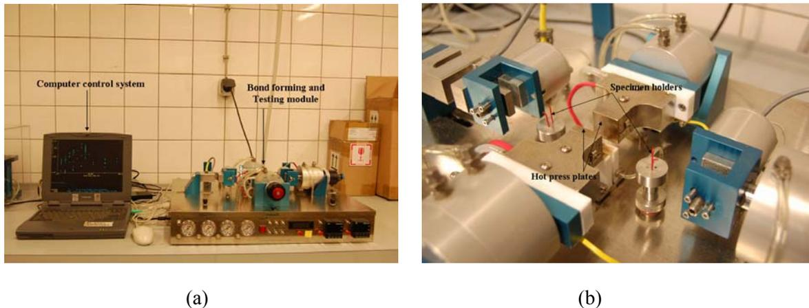
**Figure 2** Details of Automated Bonding Evaluation System device, (a) An overview of the ABES system, which is composed of the bond-forming and testing module and computer control system (b) A close-up of the bond pressing zone, which is composed of the hot press plates and specimen holders.
