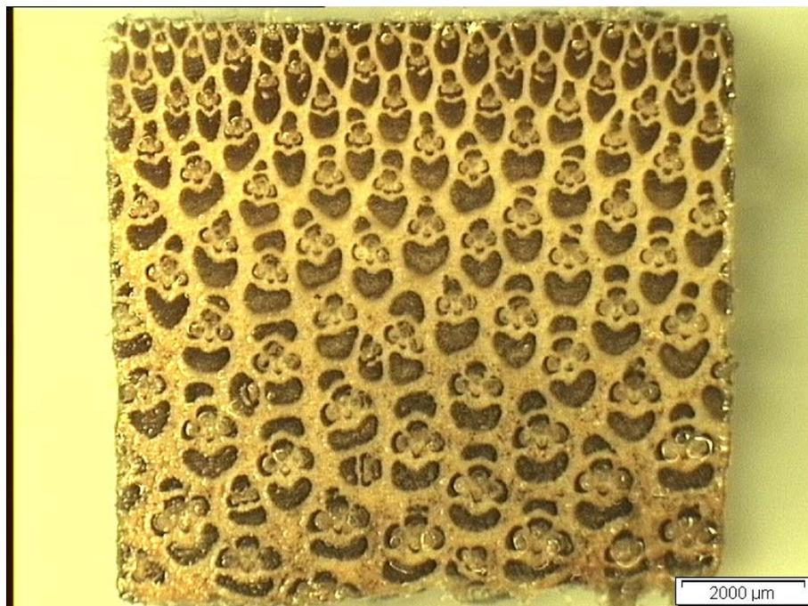
Figure 2.2 Cross section of *D. asper* culm
