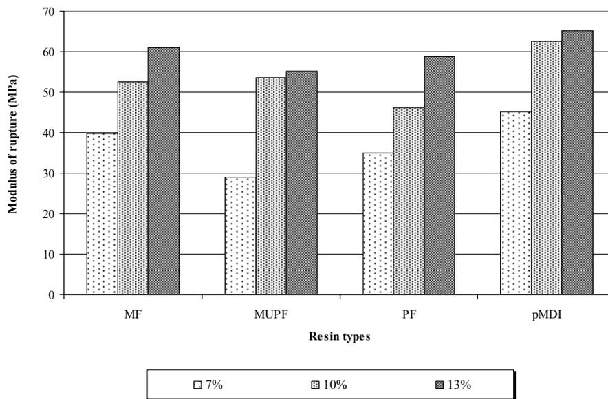
Fig. 4 Modulus of rupture of bamboo-based OSL
