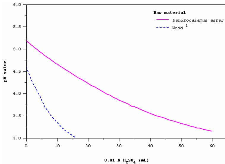
**Figure 4** The pH changes of *Dendrocalamus asper* and wood during the acid addition. Data source: <sup>1</sup> Sauter 1996
