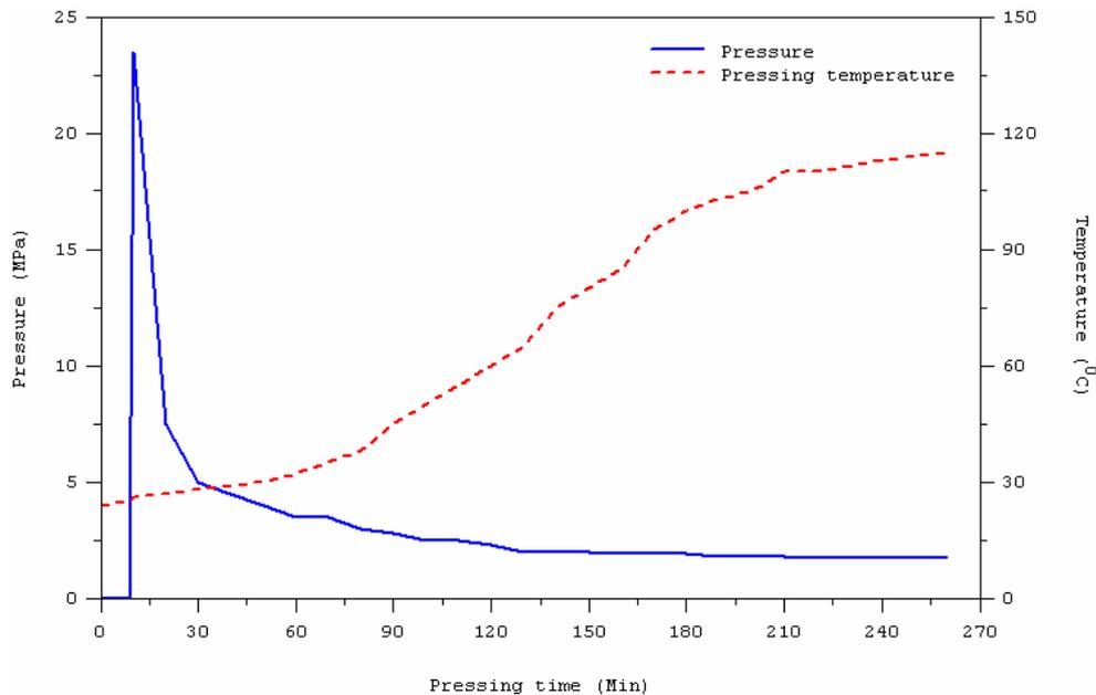
Figure 3.2 Sample of pressing diagram for bamboo-based OSL bonded with MUPF resin
