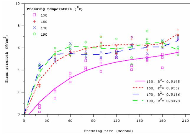
Figure 6 Development of shear strength of PF glued bamboo strands tested by ABES method as a function of pressing times and temperatures.
