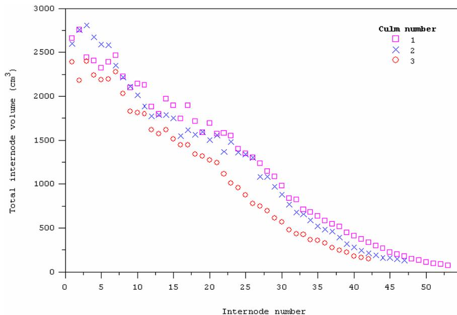
Figure 4.1 Decreasing of the internode volume of each internode along culm length of *D. asper*.
