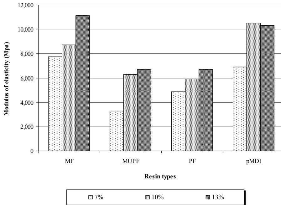
**Fig. 5** Modulus of elasticity of bamboo-based OSL
