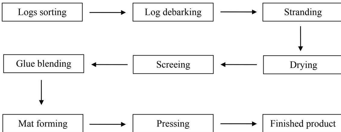
Figure 2.3 The Oriented Strand Lumber manufacturing process
