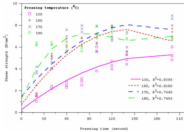
Figure 4 Development of shear strength of MF glued bamboo strands tested by ABES method as a function of pressing times and temperatures.
