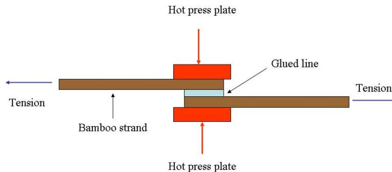
**Figure 3** Schematic description of shear test by Automated Bonding Evaluation System (ABES)
