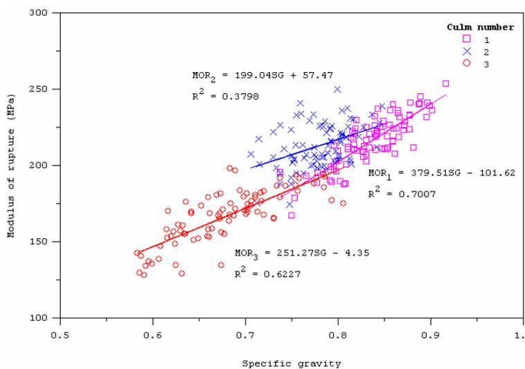
Figure 2. Correlation of specific gravity on modulus of rupture and of *D. asper*
