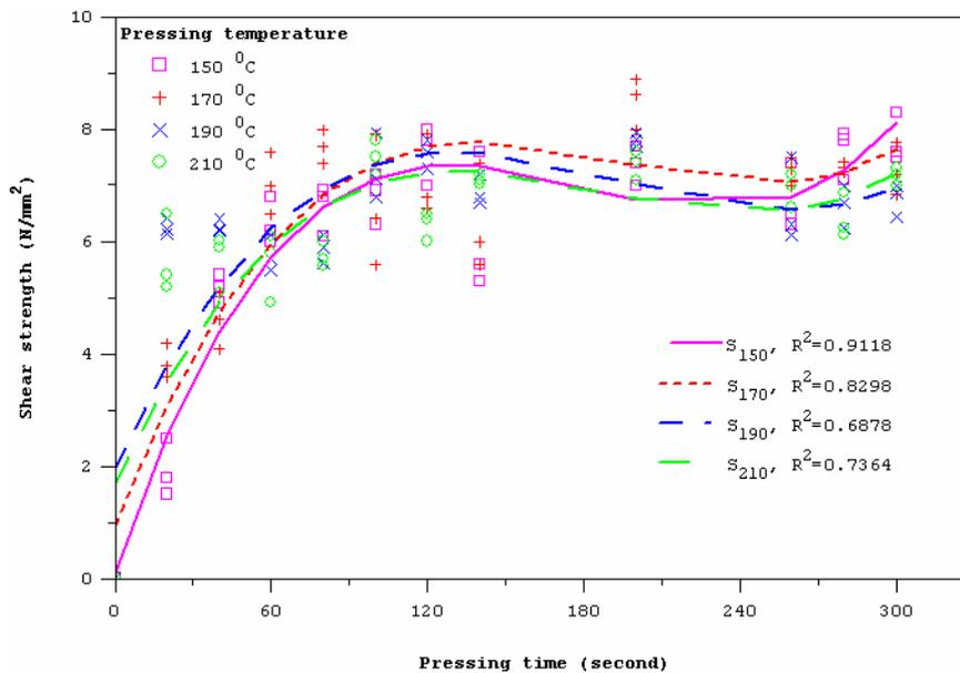
**Figure 5** Shear strength developments of MF glued bamboo strands as a function of pressing times and temperatures.
