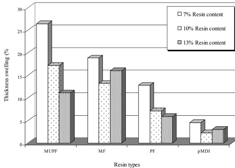
Figure 1 Effect of resin type and content on thickness swelling after 24h water soaking (20°C) of bamboo-based OSL
