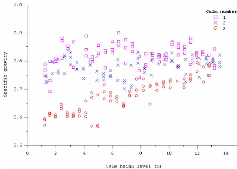
**Figure 4.** Variation of specific gravity along the culm of *D. asper* (12% MC)
