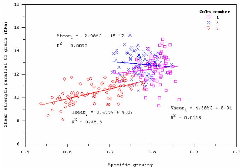
**Figure 8.** Correlation of specific gravity on shear strength parallel of *D. asper*
