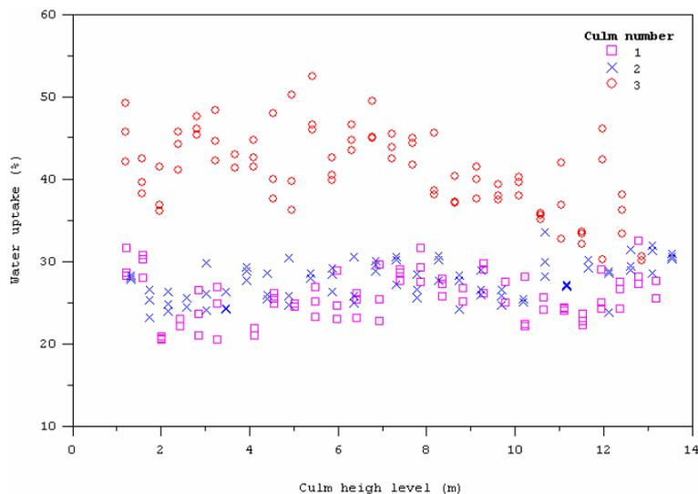
**Figure 8.** Variation of water uptake along the culm of *D. asper* (start at 12 per cent MC after 24 hrs soaking in water at 20°C).
