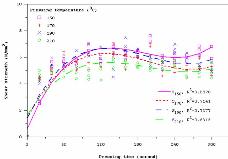
**Figure 7** Shear strength developments of PF glued bamboo strands as a function of pressing time and temperatures.
