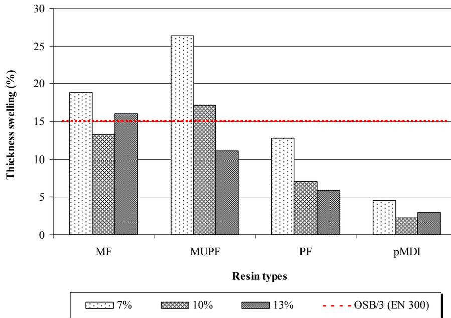
**Fig. 2** Thickness swelling after 24h water soaking (20°C) of bamboo-based OSL
