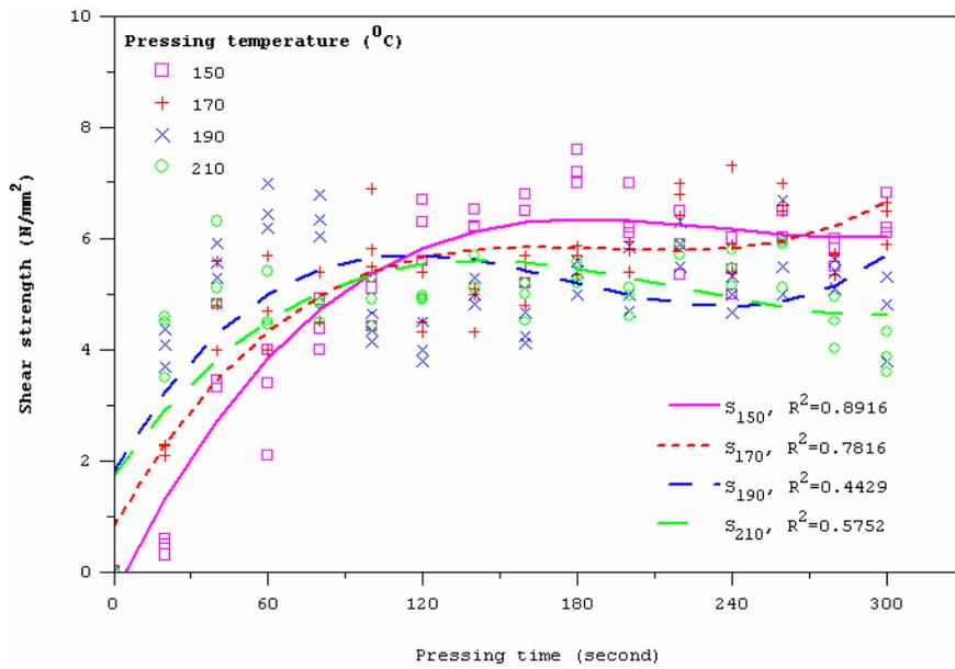
**Figure 6** Shear strength developments of MUPF glued bamboo strands as a function of pressing time and temperature.
