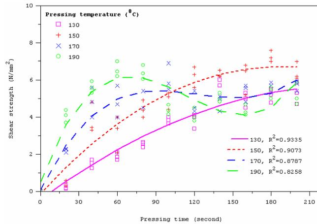
Figure 5 Development of shear strength of MUPF glued bamboo strands tested by ABES method as a function of pressing times and temperatures.
