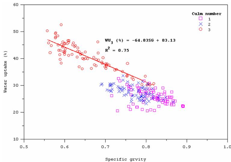
**Figure 9.** The relation between water uptake and specific gravity of *D. asper*. (start at 12% MC after 24 hrs soaking in water at 20°C)
