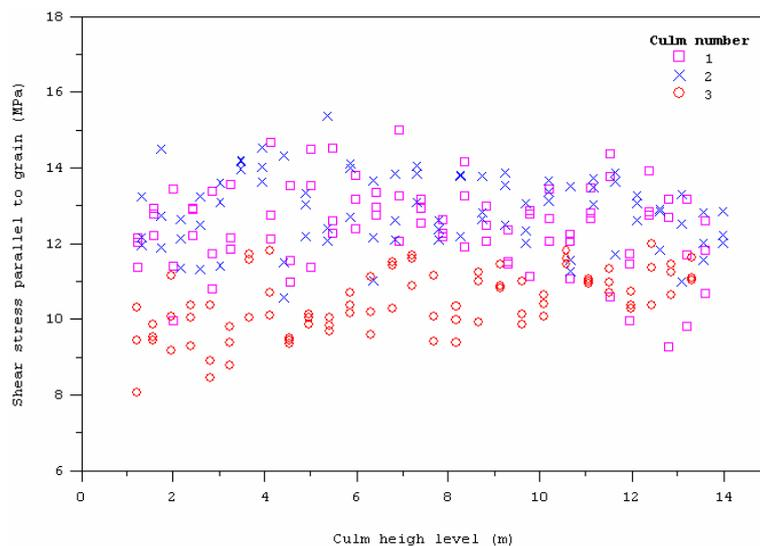
**Figure 7.** Variation of shear strength parallel to grain along the culm of *D. asper*
