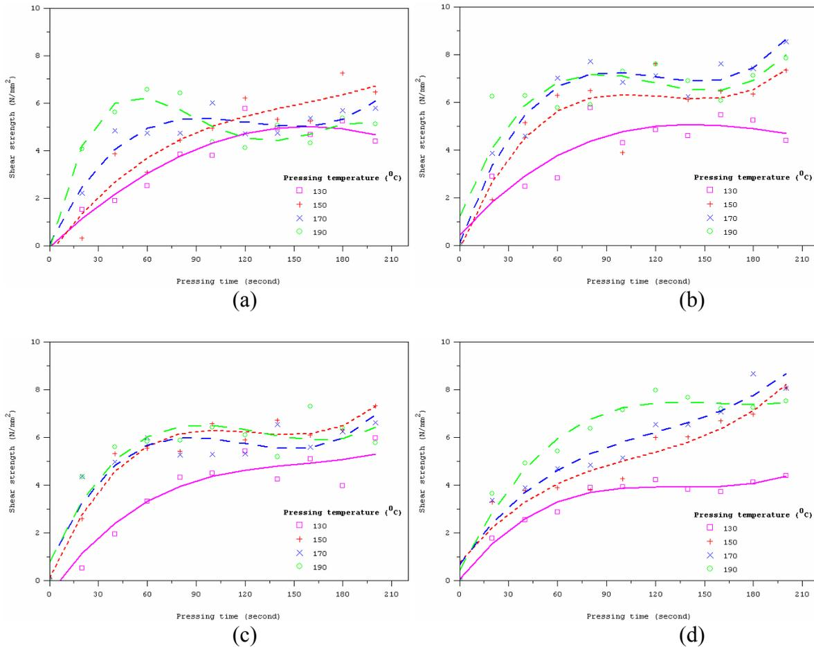
**Figure 2** Shear strength development of bamboo strands glued with; (a) MUPF, (b) MF, (c) PF and (d) pMDI, as a function of pressing times and temperatures.
