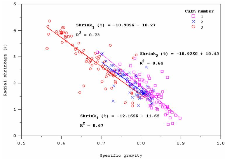
Figure 6. The relation between radial shrinkage and specific gravity of *D. asper*
