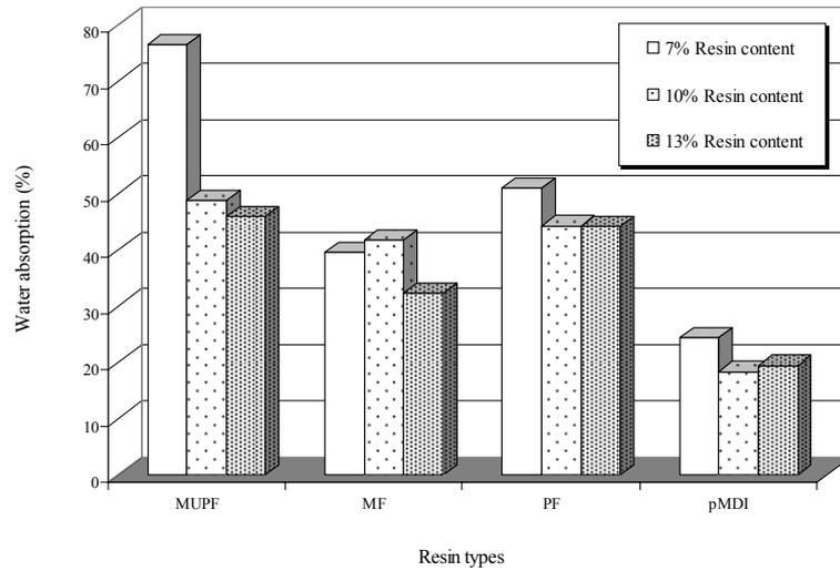
Figure 2 Effect of resin type and content on water absorption after 24h soaking of bamboo-based OSL
