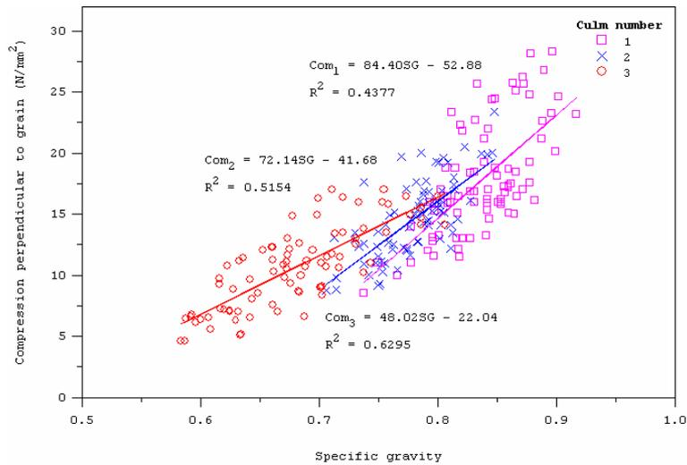
**Figure 6.** Correlation of specific gravity on compression strength perpendicular to grain of *D. asper*
