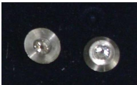
Figure A.4 Diamond anvils mounted in steel for protection and secure fixing within the cell.
