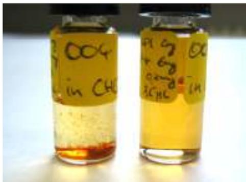
**figure 63:** FeO nanoparticles in uncrosslinked (left) and crosslinked (right) PI-*b*-PEO-OH micelles in chloroform.
