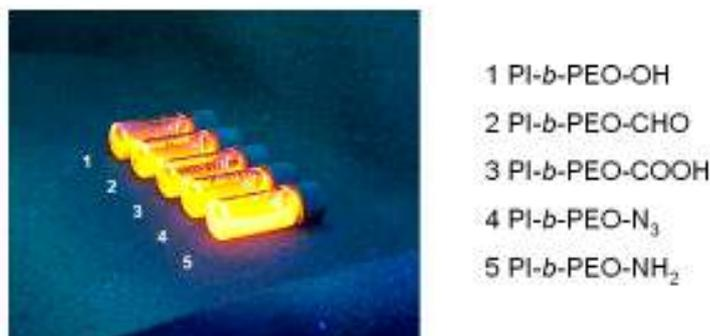
**figure 106:** For toxicity tests applied 1  $\mu$ M solutions (DMEM + 10% HEPES) of CdSe/CdS/ZnS multishell quantum dots with different PI-*b*-PEO ligand shells under UV light excitation. The solutions were previous dialysed two days to remove any salts from the nanoparticle synthesis as well as further contaminations. All solutions were autoclaved.
