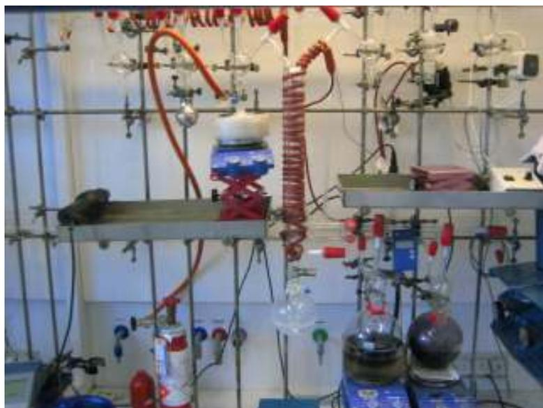
**figure 139:** cohesive glass apparatus for anionic polymerisation.
