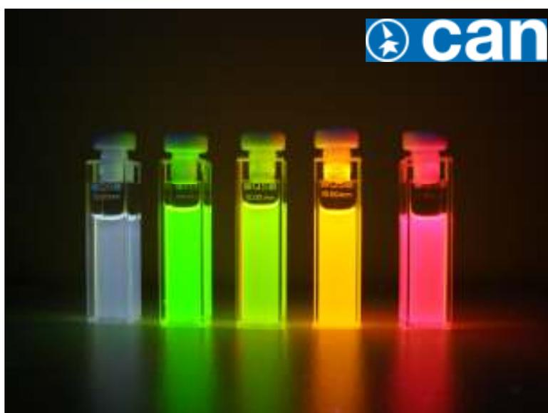
**figure 1:** CdSe/CdS core/shell nanoparticles (CAN dots) of different sizes under UV excitation.
