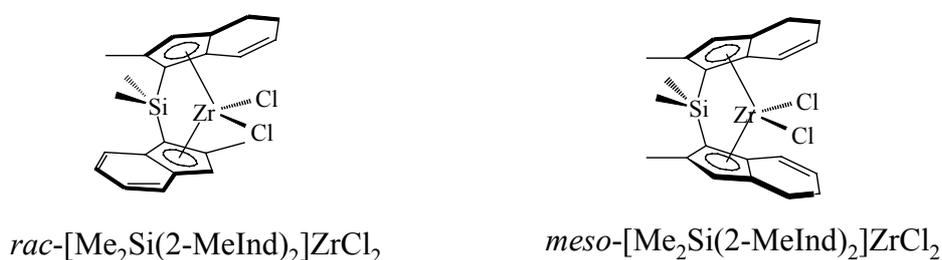
Figure 3-5: *Rac*- and *meso*-isomer of the used bisindenyl metallocene.
