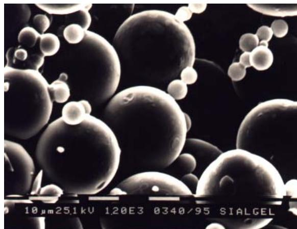
**Fig. E5.** Spherical  $\text{Al}_2\text{O}_3$  and  $\text{SiO}_2$  (x 1200)
