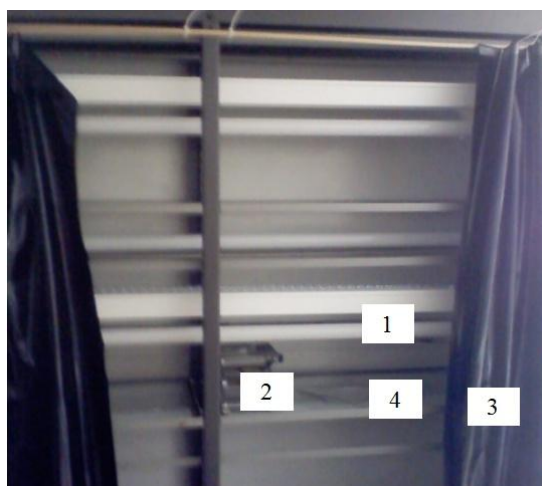
Fig. 45: A simple setup of the fluorescent lamps chamber. 1 are the fluorescence and the daylight tubes side by side; 2 is the step-up ladder where the petri dish containing the samples was mounted; 3 is the black-curtain acting as a screen; and 4 is an example of the cut-off filter used.
