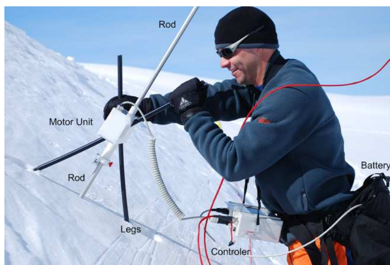
Figure 2.4: SnowMicroPen during sampling. See text for detailed explanation.
