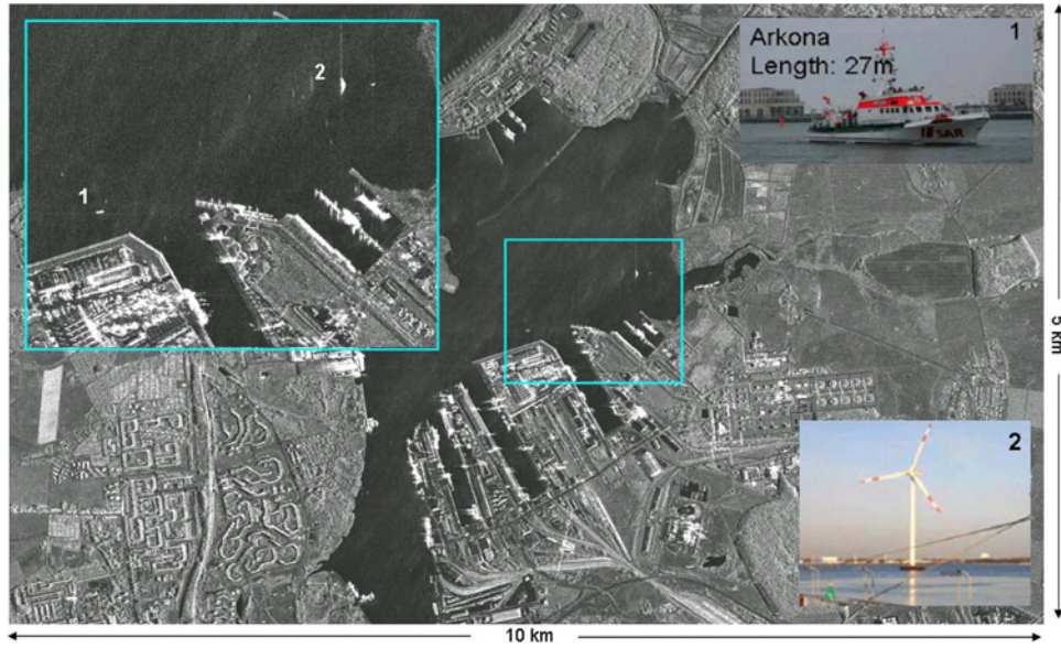
Fig. 8. TS-X high-resolution Spotlight (5 km \times 10 km, HH polarization) acquired on July 20, 2008 over the port of Rostock (Germany). (Cyan rectangle) Subscene with the SAR (Search and Rescue) vessel Arkona and a wind turbine.
