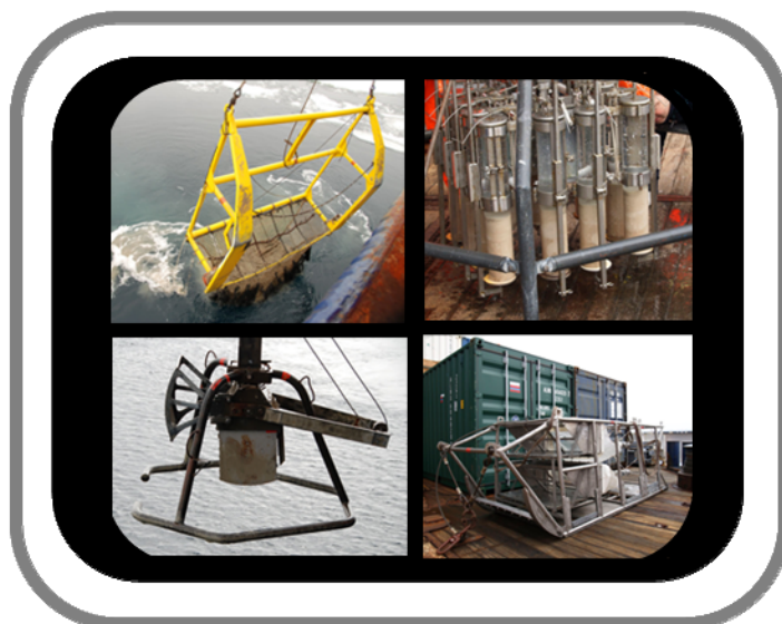
Gear used for sampling of macrobenthic organisms during the ANDEEP-SYSTCO cruise. Upper left: Agassiz Trawl, lower left: box corer; upper right: multiple corer; lower right: epibenthic sled.
