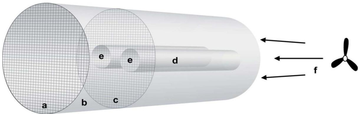
**Figure 4.1:** Wind tunnel olfactometer. **a.** gauze cover; **b.** experiment chamber; **c.** vertical gauze testing screen; **d.** glass substrate tubes; **e.** test sectors; **f.** airflow (Peters & Abraham 2009).
