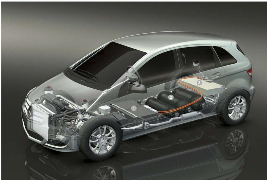
**Figure 1.2.** The Mercedes-Benz B-Class F-CELL as an example for a prototype fuel cell car. The sketch shows the most important technical features: 1 = stack of fuel cells; 2 = compressed-gas hydrogen storage system; 3 = auxiliary lithium-ion battery; 4 = electric motor. Figure reproduced with permission of Daimler-Benz AG. (15)
