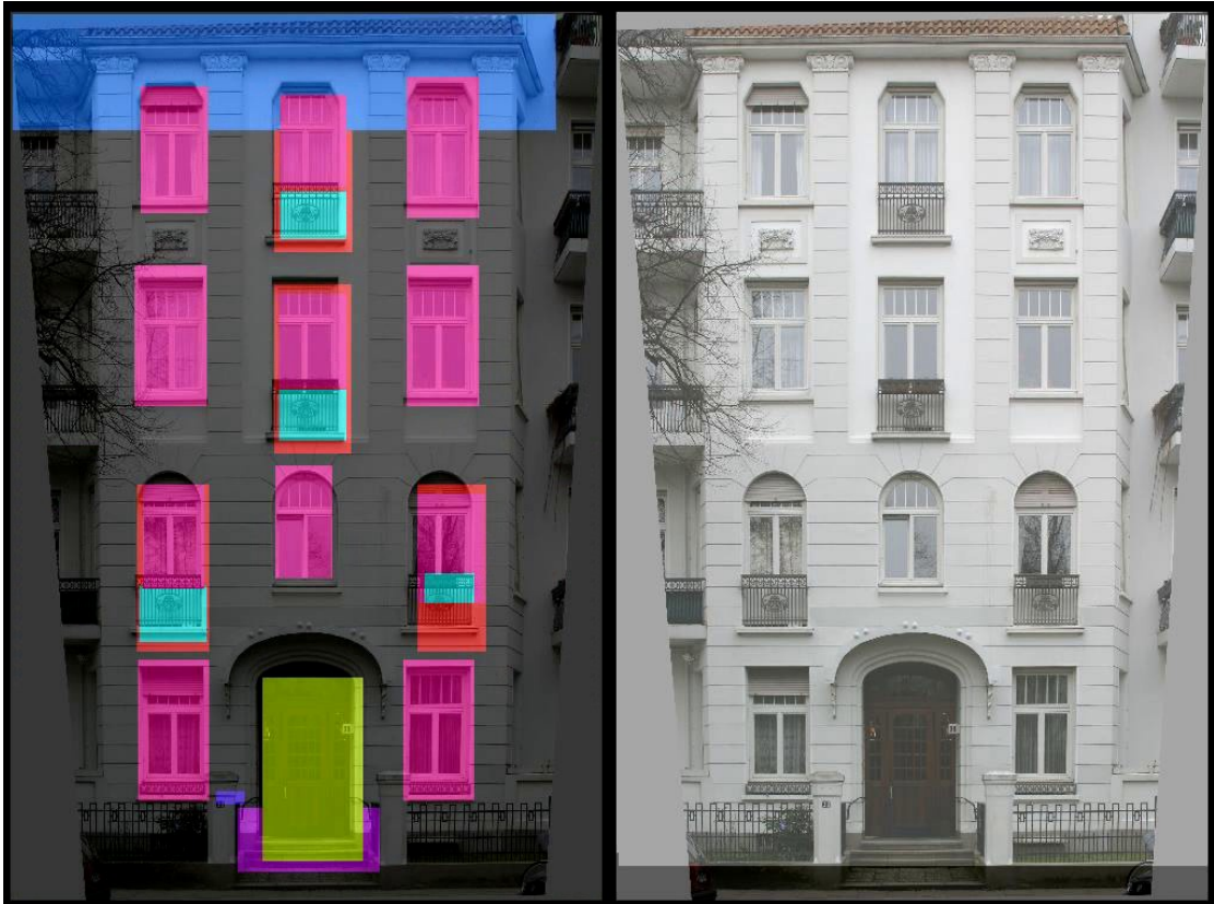
FIGURE 5.20: The result of context-based segmentation. The BCH used six structural models, out of which the most fitting one was automatically selected and used to interpret the soup of polygons provided by the low level.
