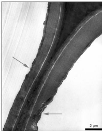
Fig. 6: Innermost part of a foundation pile with beginning cell wall erosion by bacteria [↑]. The degradation process starts from the lumen side and proceeds in direction of the S2.
