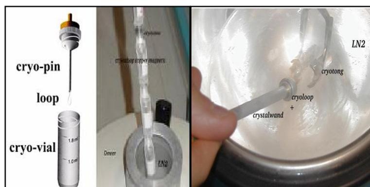
**Figure 11: Cryogenic technique accessories.**
