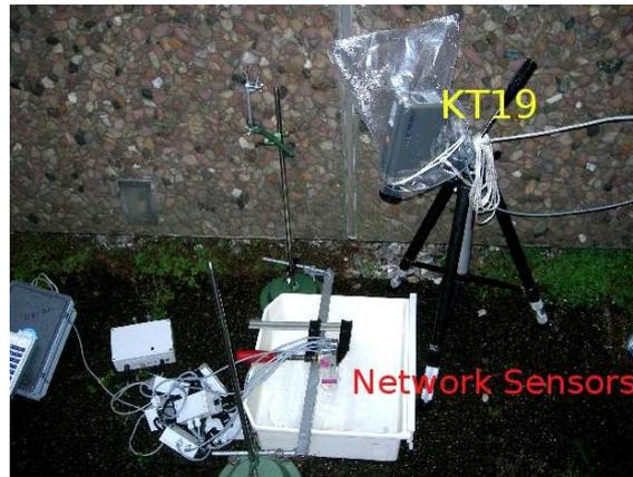
**Figure 3.5:** Calibration set-up for TNX901 Sensors. The network sensors are facing a water bath. The *KT19* used as a reference stands on the right side.
