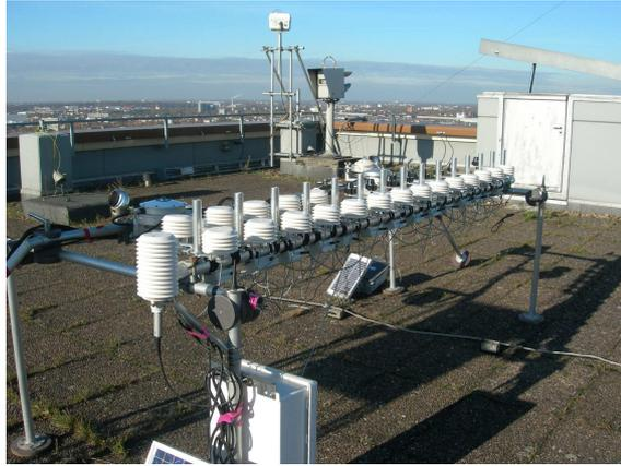
**Figure 3.1:** SHT75 Humidity and Temperature Sensors on the rooftop of the Meteorological Institute during the calibration period. The reference sensor is attached at front of the pole.
