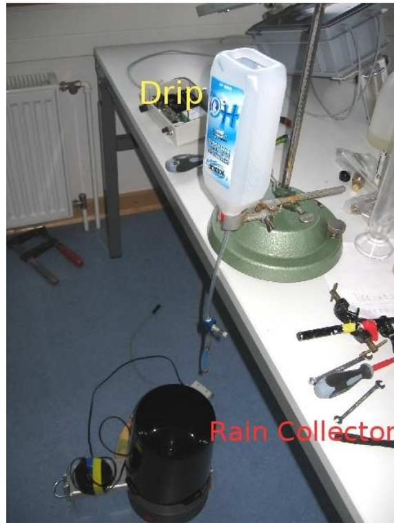
**Figure 3.10:** *Rain Collector instalment: The rain collector is placed underneath a bottle filled with 10 mm water that functions as a drip.*
