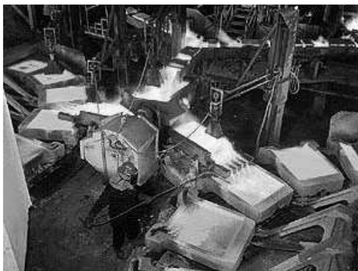
Figure 6.6: Copper from the anode furnace is cast into moulds to form anodes for the electrolysis. Source: [45].
