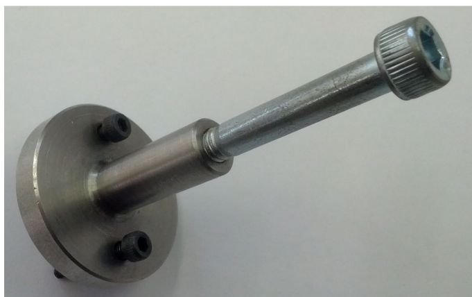
Figure A.6: Tool to open the HTHP-DAC after the experiment.
