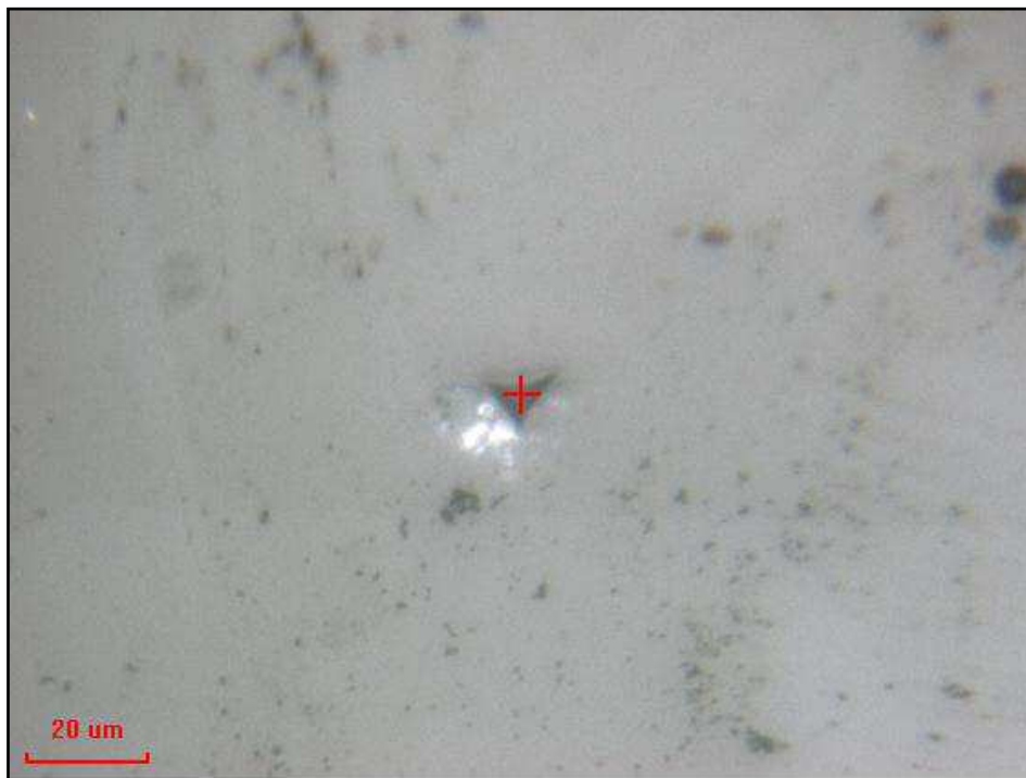
Figure 29: Optical micrograph of a nanoindent performed at RT in nonmetamict titanite from Rauris (Rauris titanite).
