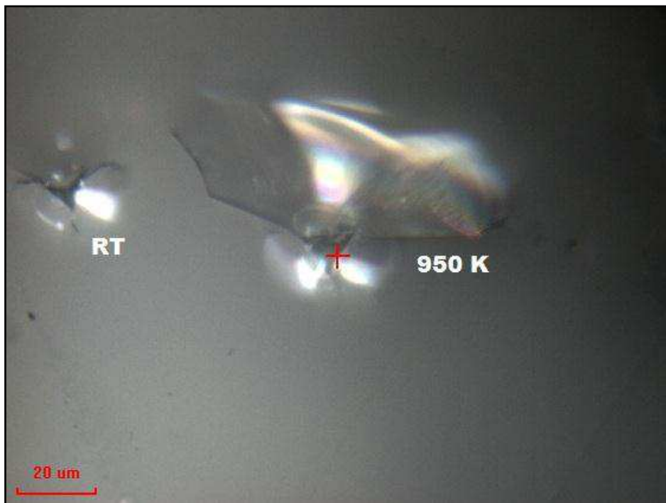
Figure 25: Optical micrograph of nanoindentations performed each time at RT in E2312 metamict titanite; unannealed (RT) and after 2 h annealing at 950 K respectively.
