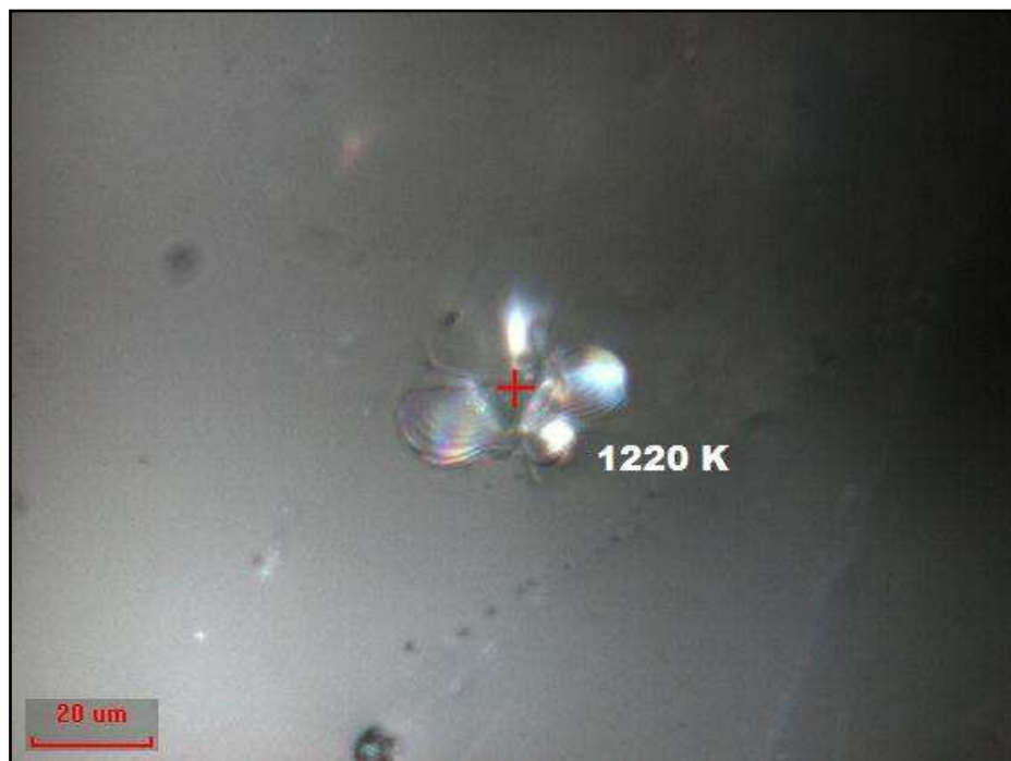
Figure 27: Optical micrograph of nanoindentations performed each time at RT in E2312 metamict titanite; after 2 h annealing at 1220 K.
