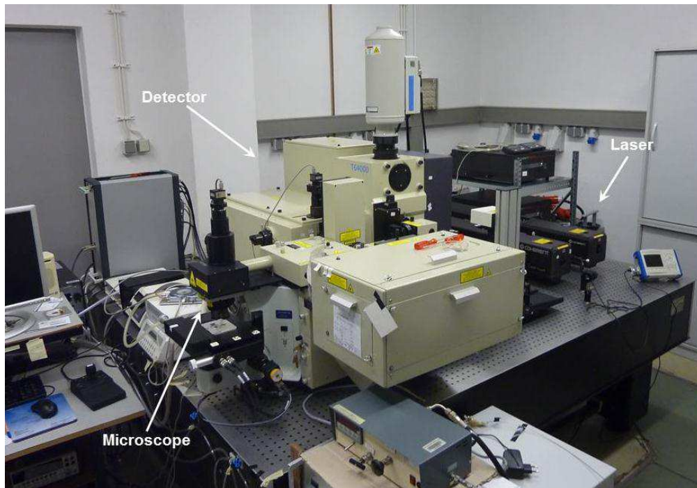
Figure 5: Raman spectrometer: Horiba Jobin-Yvon T64000 triple monochromator system, equipped with a liquid N 2 -cooled charge-coupled device (CCD) detector and an Olympus BH41 microscope. The laser is an Ar + -ion laser.
