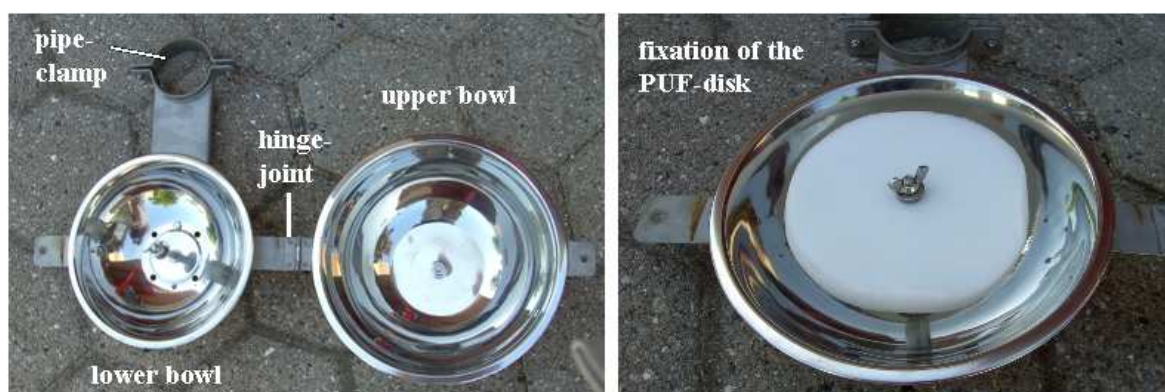
Figure 3.7: Modified PUF disk passive air sampler
