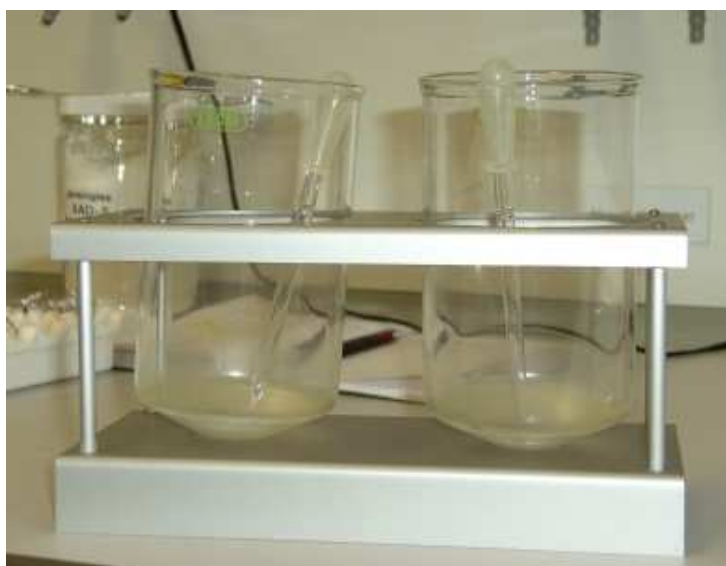
Figure 4.21: Glass jars of the parallel-evaporator system glazed with tenacious PUF residues
