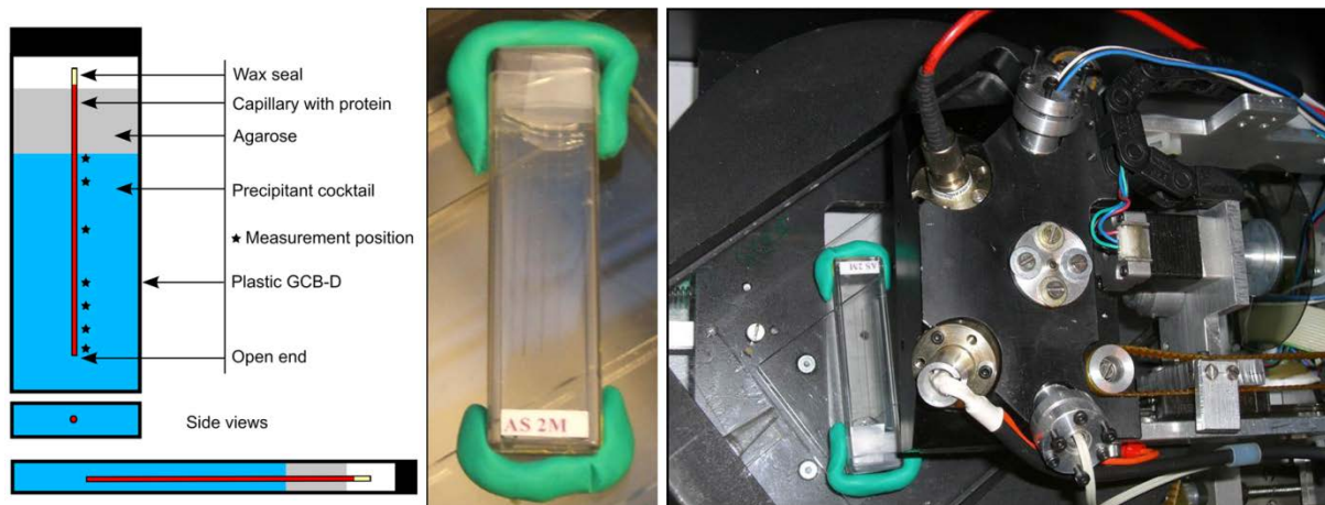
Figure 8: Schematic drawing and figure of a GCB-D alone and inside the SpectroLIGHT 500 . A schematic set up of a counter-diffusion experiment is shown on the left side. The open end of the capillary allows the precipitant to diffuse against the much slower diffusive protein solution, thereby inducing the precipitation of the protein. Each mark (*) represents a DLS measurement position, at 0.7, 2.2, 5.1, 9.9, 11.8, 18.7 and 24.5 mm from the open end. In the middle a GCB-D used for in situ DLS experiments is shown and on the right side a GCB-D within the SpectroLIGHT 500 is shown.
