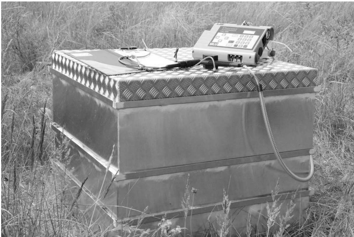
Figure 17: Stationary chamber with inserted additional frames and mobile FID during measurement.
