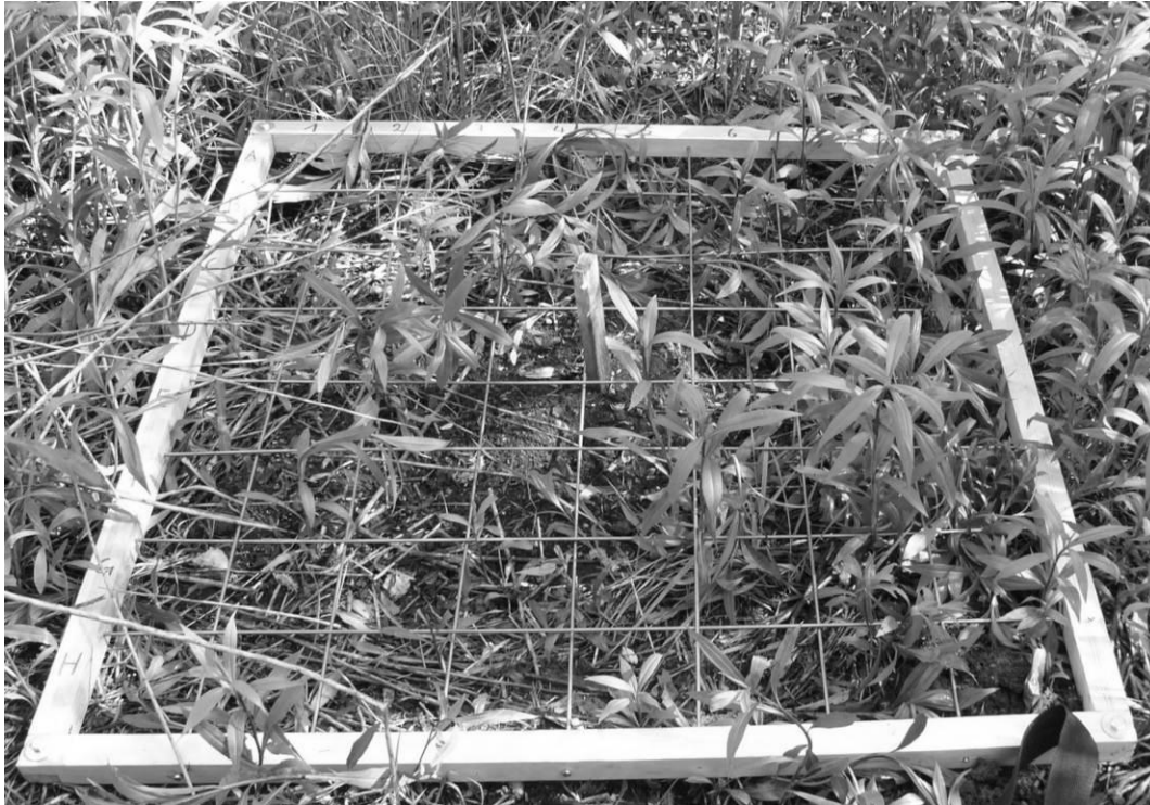
Figure 16: Frame with grid used for measurement of small-scale variability of methane surface concentrations on landfill H. The stake marks the location of the hotspot emission measurements.
