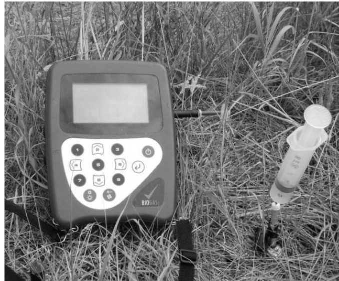
Figure 13: Sampling and analysis of soil gas probes
