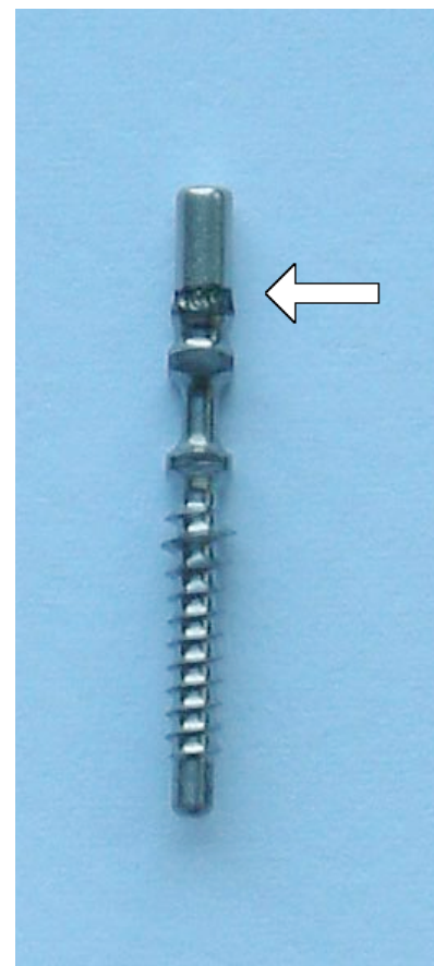
Fig. 1. Neodymium magnet laser spot welded onto the temporary implant, over all length 20.8 mm. Arrow indicates welding suture.
