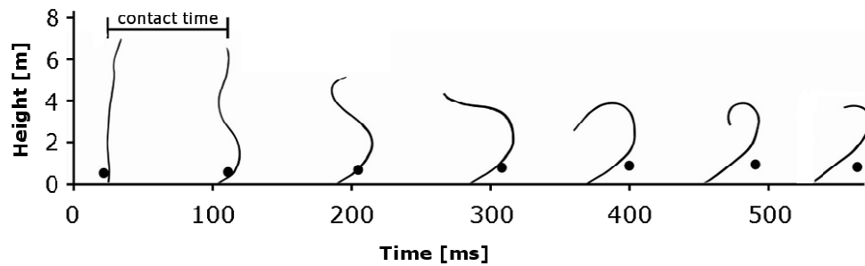
Figure 3.5: Demonstration of the flexural deformation of an entire coppice tree during and after bob impact (total tree height: 8.3 m; stem height (with diameter > 0.025 m): 6.5 m; DBH = 0.05 m). Each of the seven sketches depicting stem and bob shape is extracted from high-speed camera images.
