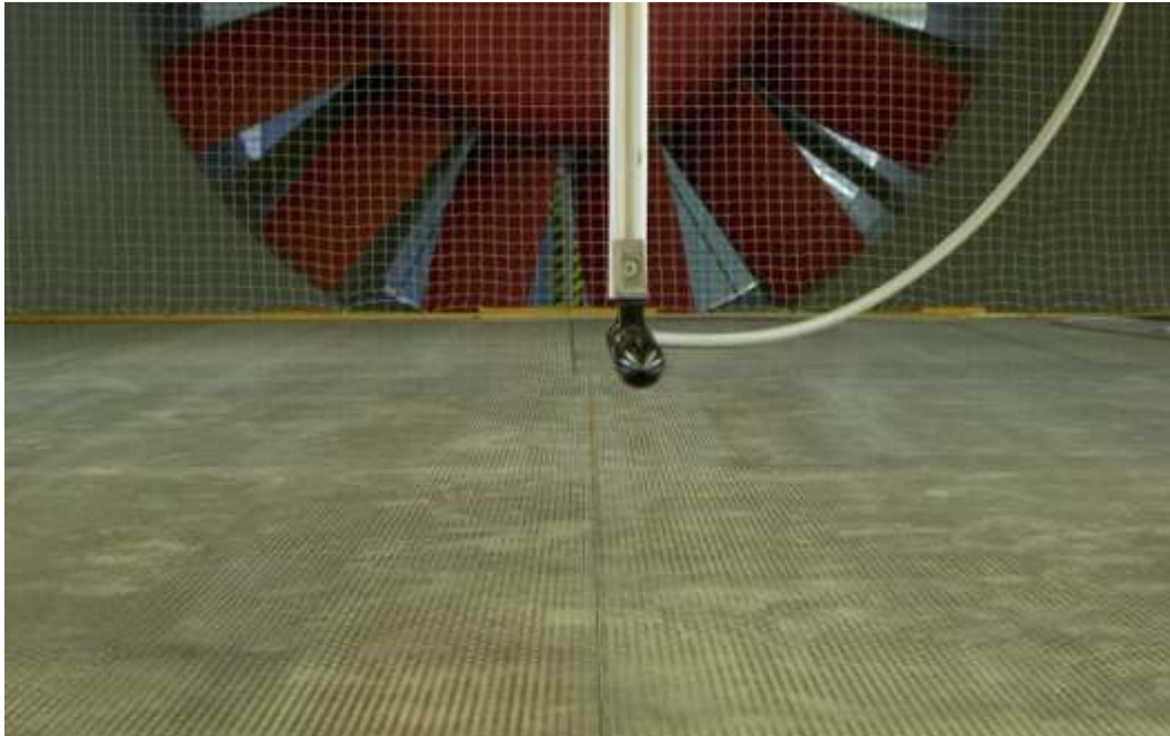
Figure 52: Bolund study laser-doppler-anemometry (LDA) probe and empty model area. Credit: Stephan Werk
