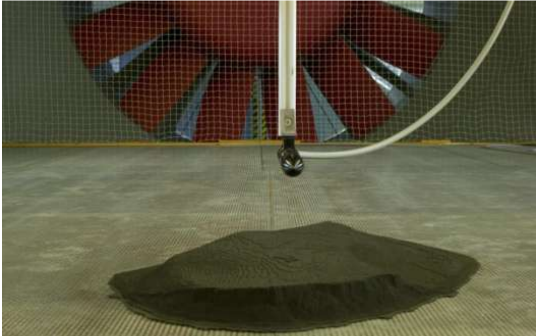
Figure 55: Bolund hill model in 1:250 and LDA probe in wind tunnel WOTAN. Credit: Stephan Werk
