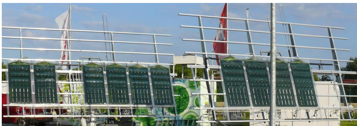
Fig. 1 Outdoor system used in present study equipped with solar tracked PBRs and a temperature control by cooling and heating. Flue gas from a power plant was used as the only CO 2 source for the microalgae production.
