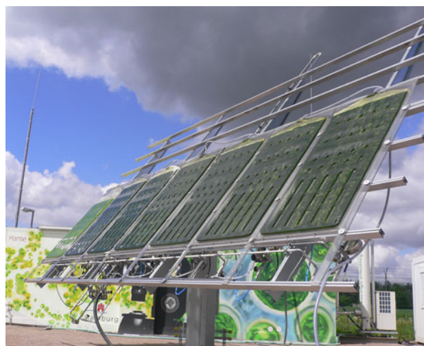
Fig. 1 Flat panel photobioreactors mounted on a solar tracker. The optical light path of the PBRs varied between 15 and 22 mm
