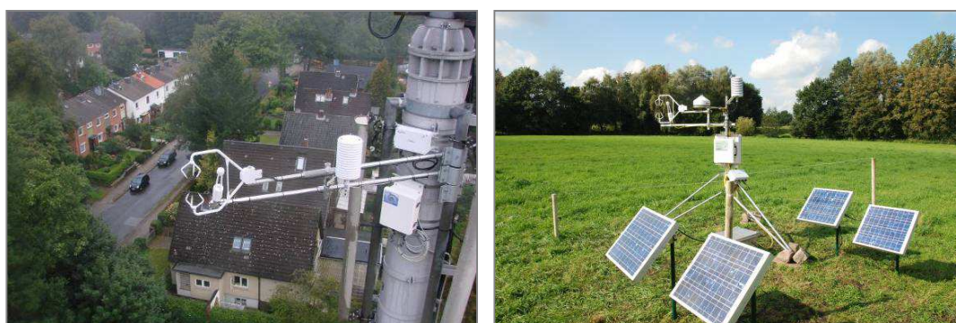
Figure 3.5 Eddy covariance systems at SGD (left) and DGD (right).
