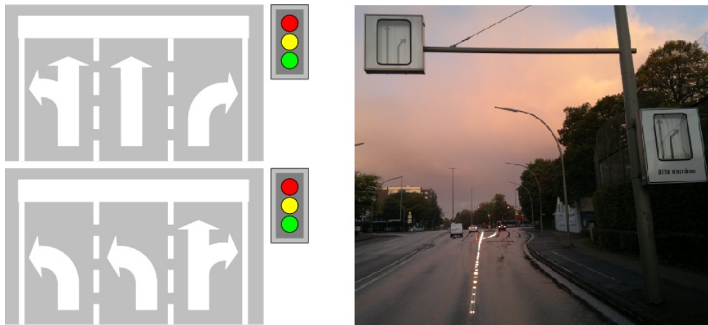
Figure 7.3 – Dynamic lane allocation: examples of how flows may be allocated to lanes [from Göb08a, p. 9] (left) and a traffic sign displaying the current lane allocation (right)
