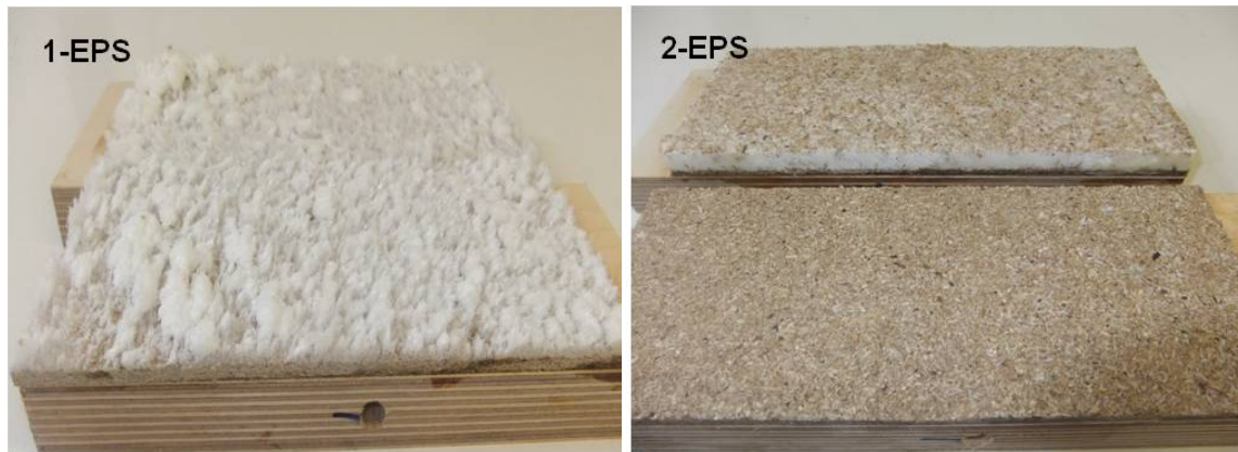
Figure 11: Failure made in tested foam core particleboards for planar shear test
