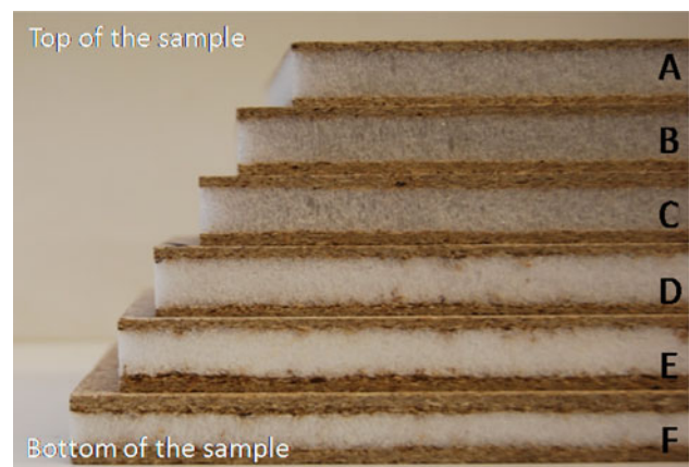
Fig. 1 Varieties of lightweight foam core panels; 1-EPS (130 °C: A, B, C) and 2-EPS (160 °C: D, E, F)
