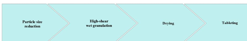
**Fig. 1:** Simplified presentation of the most important processing steps during the manufacturing of a tablet formulation (modified from [30]).
