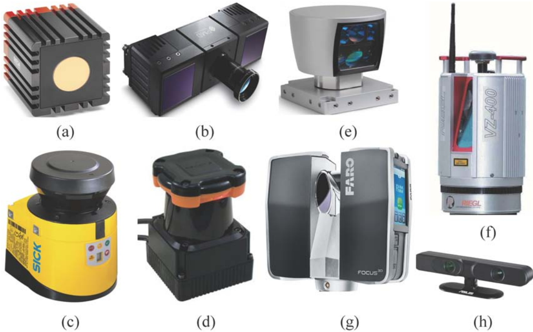
Figure 2.1: State of the art range sensors. (a): SwissRanger SR4000; (b): PMD[vision] CamCube 3.0; (c): SICK S300; (d): Hokuyo UTM-30LX; (e): Velodyne HDL-64E; (f): RIEGL VZ-400; (g): FARO Focus 3D ; (h): Asus XtionPro.
