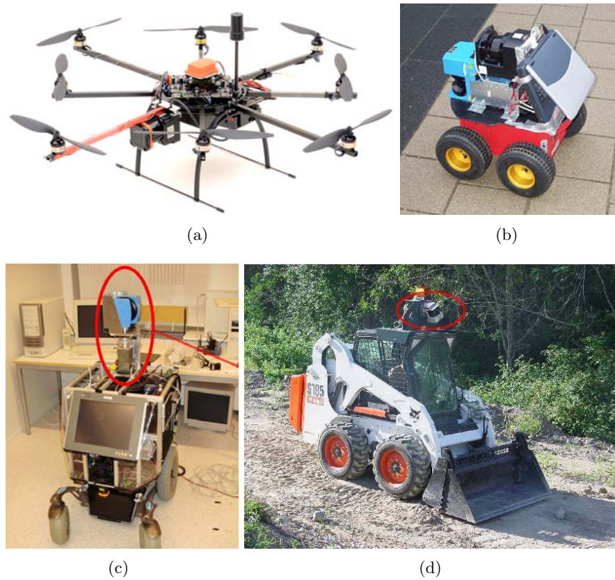
Figure 2.3: Experimental platforms have been employed for continuous 3D scanning. (a): our custom-built octocopter in Adler et al. (2012, 2013); (b) platform used in Hänel et al. (2003); (c) platform used in Stoyanov and Lilienthal (2009); (d): platform used in Bosse and Zlot (2009a).
