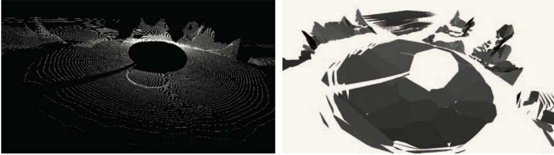
Figure 2.8: Left: a point cloud from a simulated robot with Velodyne 3D LRF in a scenario with ground-truth data from Mars. Right: Planar patches based representation of the point cloud. The figure is adapted from Birk et al. (2009).
