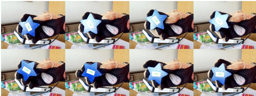
Figure 6.21: Star prism gaiting learning from human demonstration. In this scenario the demonstrator uses the thumb, first, middle, and ring fingers to anticlockwise rotate the posture of the star prism.
