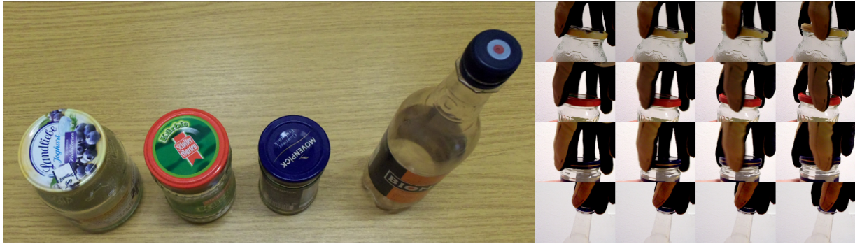
Figure 3.9: Unscrewing different-sized bottle-screw-caps. The thumb, first, middle, and ring finger participate in this scenario. Each screw cap is rotated as around 90^\circ anticlockwise, and this process is defined as a trial.
