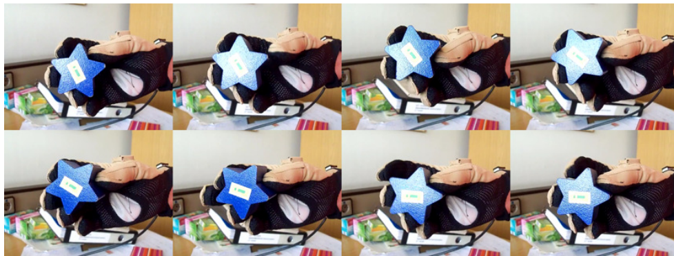
Figure 3.7: Rotating a star prism. Thumb, first, middle and ring finger are used to rotate the block. In the stable moment, four fingers pinch the grooves. For rotation, each finger reaches the neighbor groove. This process is defined as one trial, and we will see the hand pose at the beginning state is quite similar to the end state.
