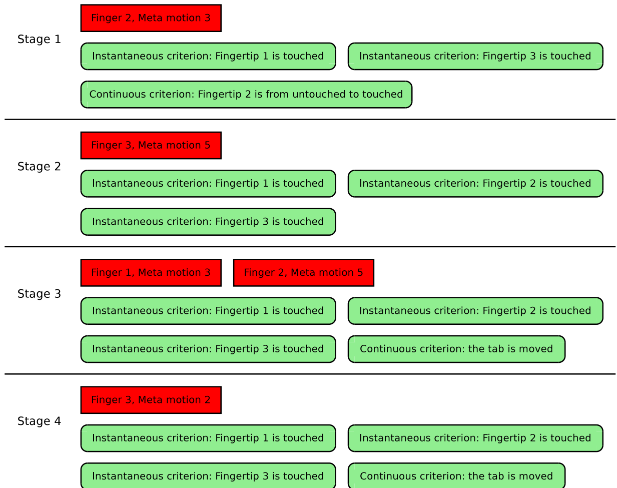
Figure 4.1: An example of state-action gist. Suppose that we are now trying to open the tab of a can with the thumb, first and middle fingers. After extraction, we have such form of meta motions and meta criteria. We should claim that there are countless methods to open a can, this example is just a case of this in-hand manipulation skill. Depending on the trigger time of the motions, we have four stages, and meanwhile we collect the meta criteria from available sensors. For the meta motions, having the start time is enough. This is because we extract meta motions sequentially; the moment that a motion starts at a finger, indicates the previous motion stops at that finger. For the meta criteria, we mark them at the moment that the next meta motion is triggered (or the end of this manipulation). In this case, the instantaneous and continuous criteria step-by-step present the necessary achievements in the manipulation task. Specifically for this example, we keep the thumb and the middle finger fixing on the can, so the contact states of these two fingers keep “in touched” in all stages. Besides, we use the first finger to open the tab on the can, so we see the first finger approaches to the can in stage 1. Last but not least, for this scenario, our aim is to open the can by moving its tab, so in the stage 3 and stage 4 we find the tab is moved.
