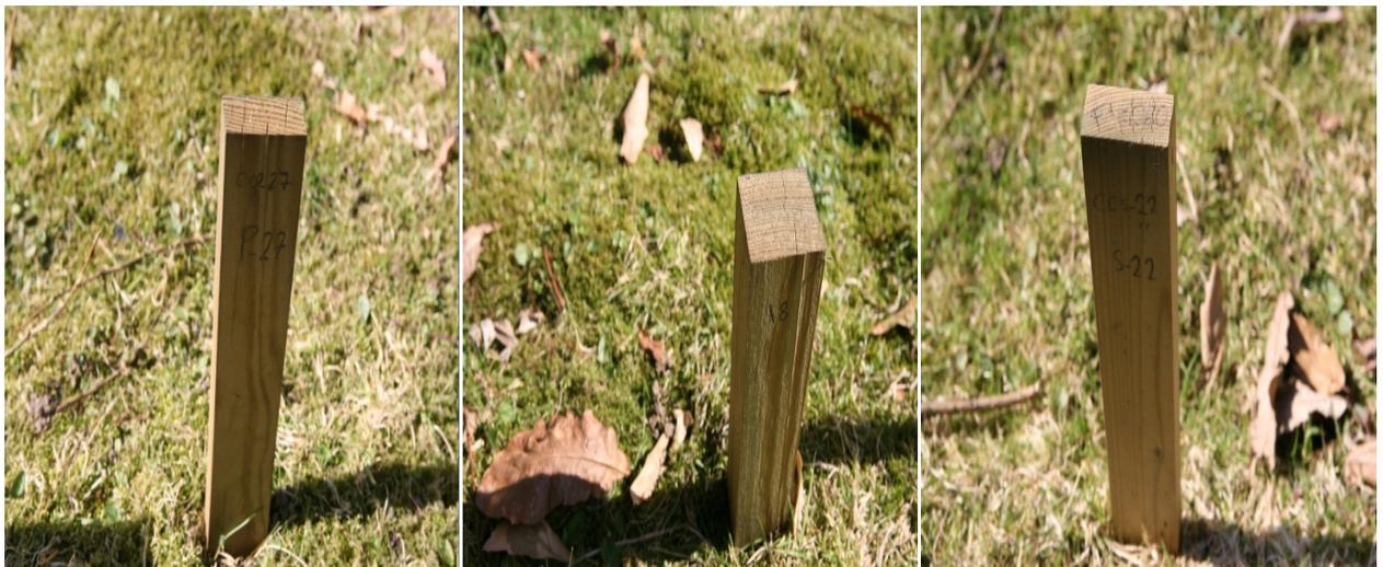
Figure 2.5: Samples of EN 252 pine sapwood (left), non-standard pine sapwood (center) and EN 252 spruce (right) to demonstrate the different sizes
