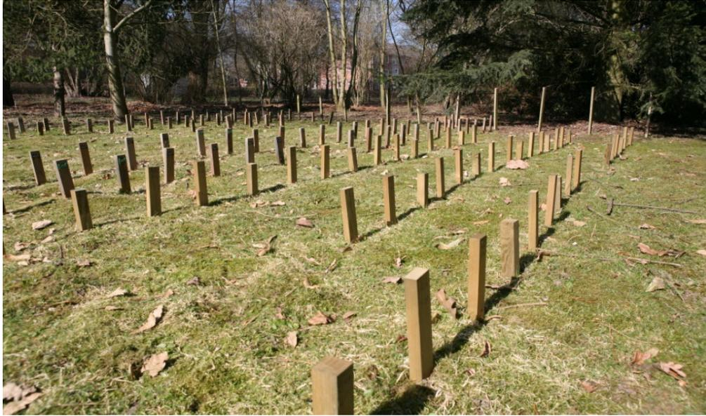
Figure 2.4: DIN EN 252-stakes and non-standard stakes installed in ground on July 30, 2010
