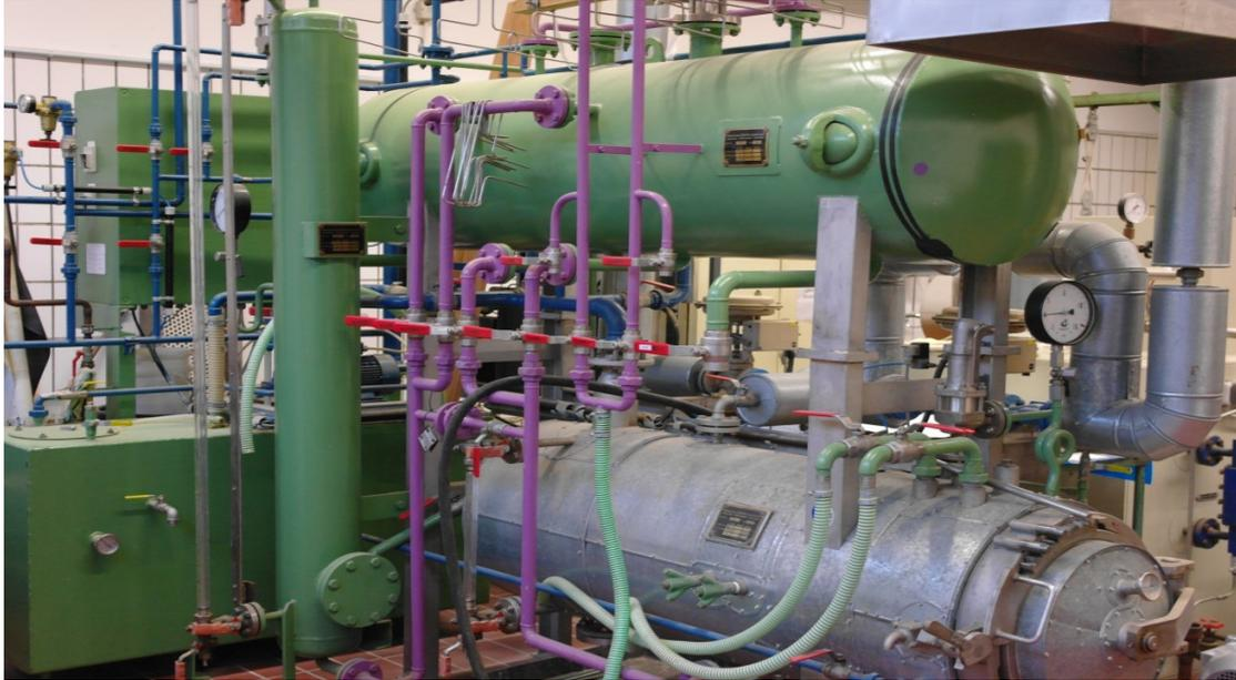
Figure 2.1: Pilot treating cylinder used for impregnation of wood samples
