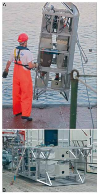
**Figure 1.** The thermo boxes on the Camera Epibenthic Sledge (C-EBS; Brandt *et al.* 2013) are able to reduce warming of the samples during retrieval through the water column. A.) While the C-EBS is veered and heaved through the water column, the lever is extended (a). The thermo boxes (b) are closed. B.) When the C-EBS is at the bottom, the lever is bushed in and the thermo boxes are thus open (c) to reduce dynamic pressure.
