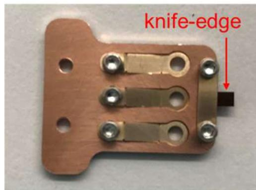
{Figure 5.9. Knife-Edge structure attached on the sample holder }
