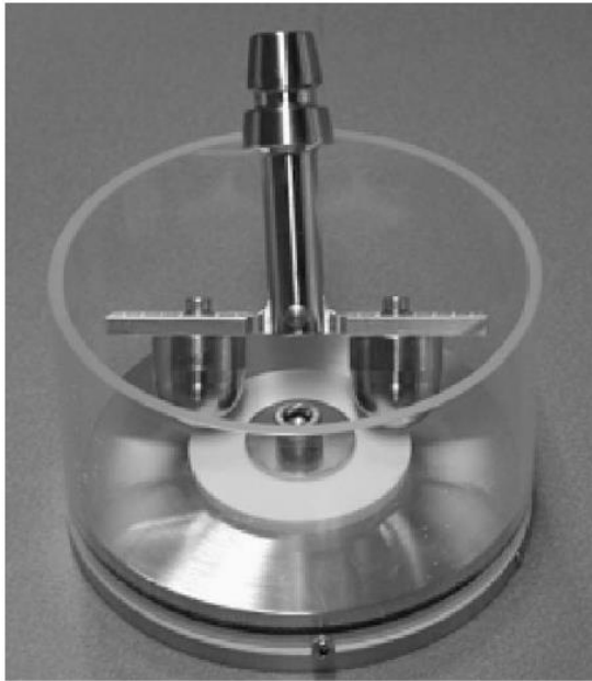
Figure 3.18 Image of the tribometer cell used in combination with Physica UDS 200 (Anton Paar GmbH) (Reprinted from Ref.[98])
