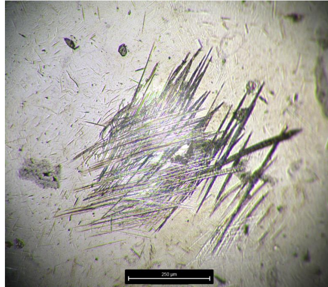
Figure A.2 Photomicrographs showing the scratches on the tips of a steel ball after the frictional measurement on the 1164D surface
