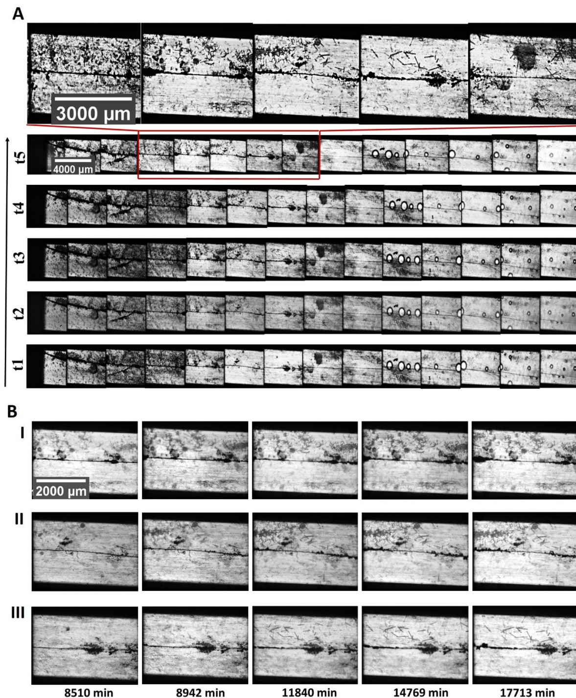
Figure 55. Protein crystallization in microgravity applying the counter diffusion technique in capillaries. Images were recorded using the ISS LMM microscope. PfGST dimer crystals. (A) Time-lapse images were recorded with 2.5 x magnification. The imaging time extended to t = 17713 min, images were taken t_1 = 8510 min, t_2 = 8942 min, t_3 = 11840 , t_4 = 14769 min and t_5 = 17713 min after sample thawing. (B) Time-lapse images were recorded for 3 different areas (I, II, III) with 2.5 x magnification.
