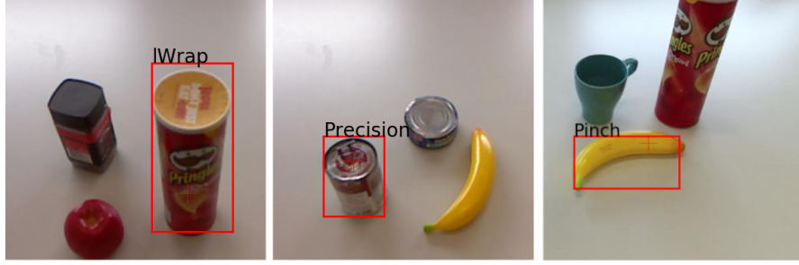
Figure 5.2: Examples of grasp-relevant information extraction. The red bounding box denotes object locations. The text denotes grasp types (here, the lWrap denotes the large-wrap ). The red cross denotes the location of the grasp attention point.
