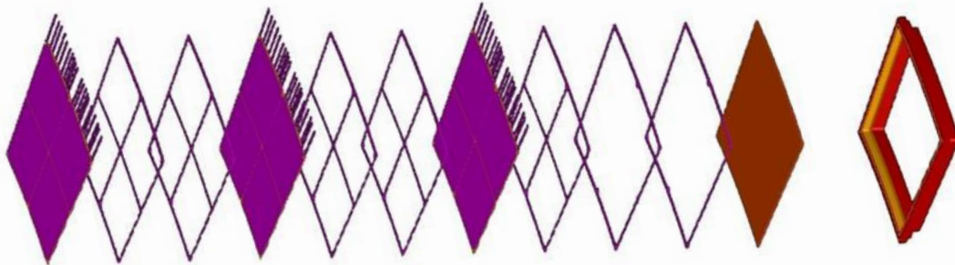
Figure 7.1: Exploded view of the GridGEM module showing the different components stacked one after the other. From the right is possible to see the back-frame, followed by the PCB, 3 ceramic components spacing the first GEM of the stack. The other 2 GEM are similarly spaced by other ceramic components including a grid shaped inner element to reduce the sagging of the foils due to the electromagnetic and gravitational forces involved.
