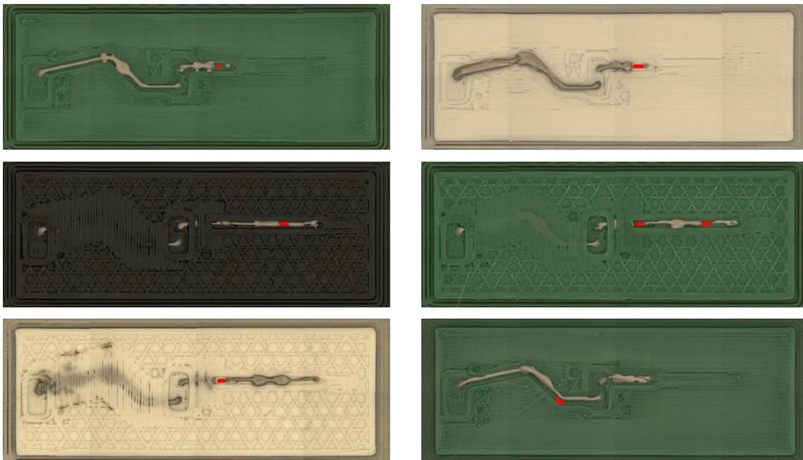
**Figure 6.9** – Objects printed with intentionally de-calibrated syringe extruder to evaluate the detector performance. Defects automatically detected by the verification algorithm are highlighted in red. For this test dataset, the algorithm detected 100 % of all defects.
