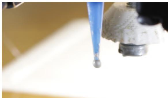
**Figure 3.11** – Oozing at the syringe extruder due to thermal expansion.
