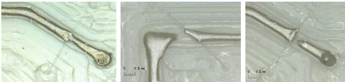
**Figure 7.1** – Partly or fully interrupted conductive traces due to stringing from the plastic extruder. The threads are barely visible with naked eye.
