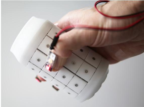
**Figure 7.8** – Can-shaped tracking object with tactile feedback.
