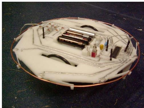
**Figure 2.1** – Prototype of a printed, mobile robot. Electrical connections are realized with low-temperature metal alloy. All circuits were manually dispensed and assembled. Reprinted image courtesy of [A73].
