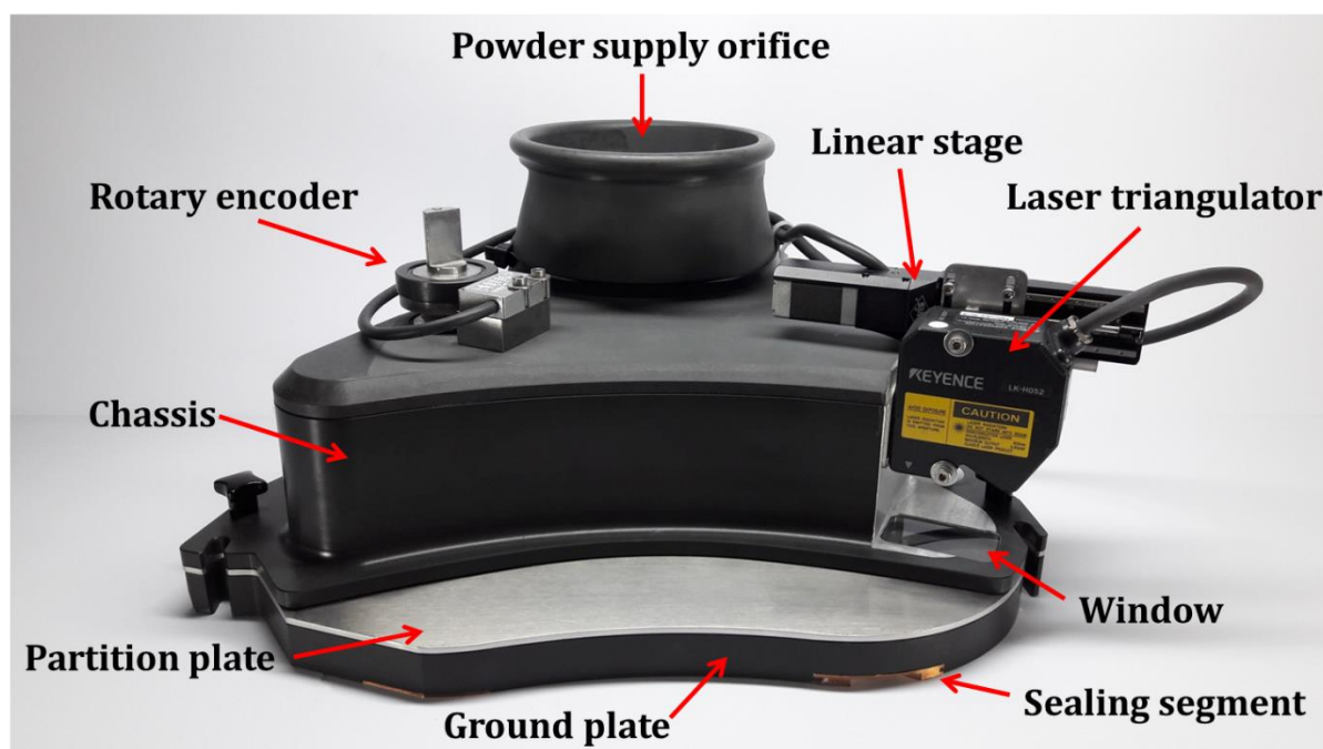
Fig. 15: Instrumented feed frame.
