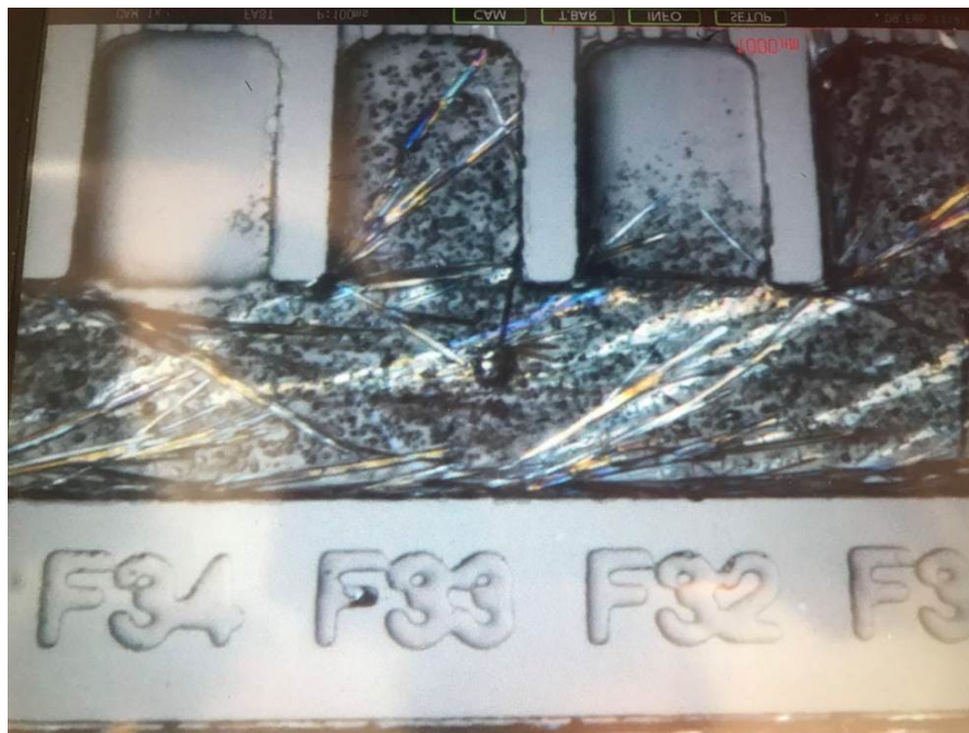
Figure 5.11: PDMS chip for crystal growth and storage.
