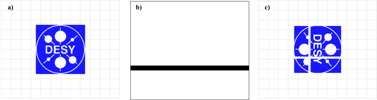
Figure 4.7: Validation of image transfer with a binary transmission mask ‘slide’ at the SLM surfaces. a) input image b) binary transmission mask c) output image
