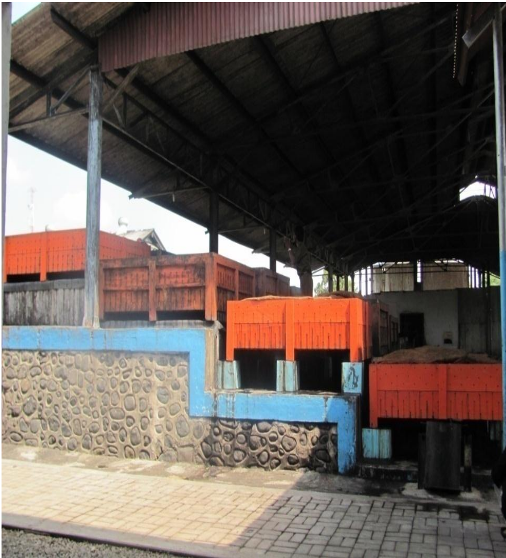
Figure 1.6 Box fermentation, capacity 800 – 1000 kg Nusantara Plantation XII (PTPN XII), East Java, Indonesia
