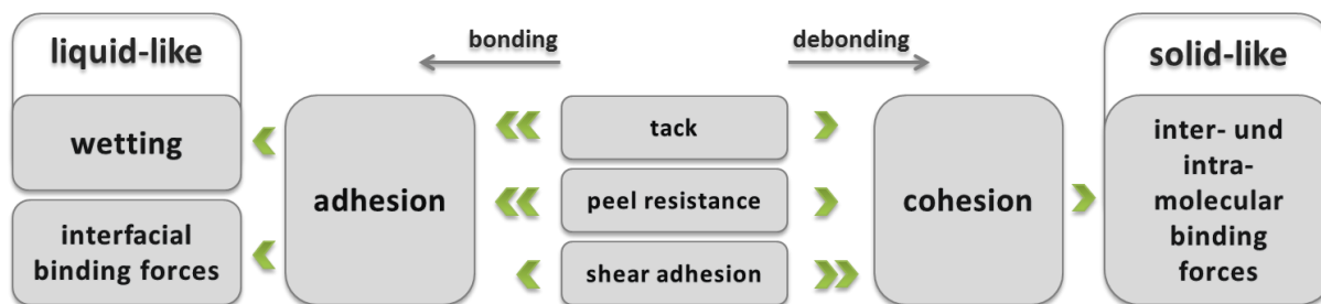
Fig. 8: Adhesion performance considering tack, peel resistance, shear adhesion and their relation to liquid- and solid-like behavior of bonding and debonding of a PSA.
