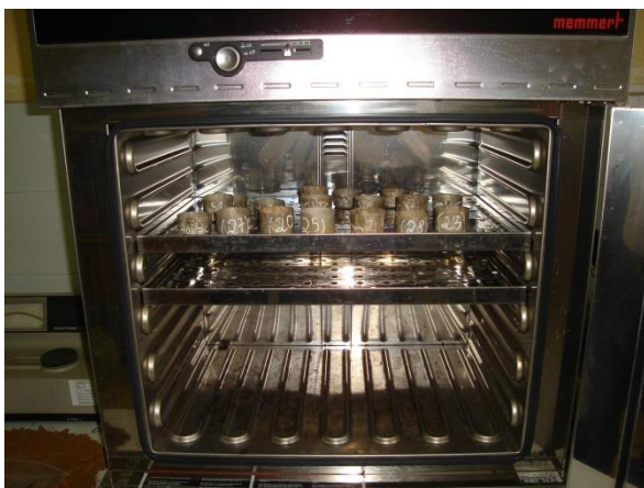
Figure 3.12 Oven drying soil sub-samples (replicates).
