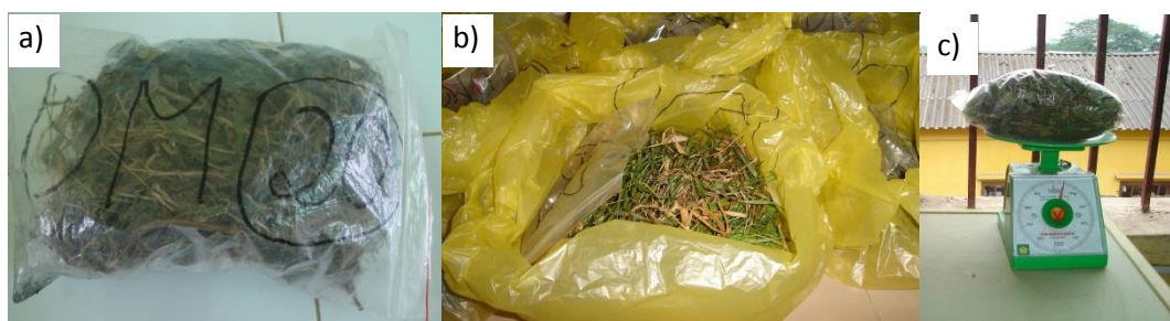
Figure 3.10 Collection and handling of understorey biomass samples: a) sub-sample preparation, weighing and labeling, b) air-drying before sending the sub-sample to lab, and c) weighing sub-sample in lab.
