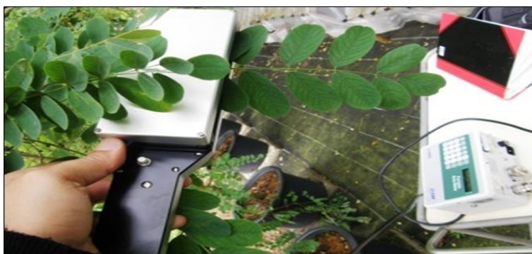
Fig. 4.8: Leaf measurements by a Leaf Area Meter (Li-Cor model 3000, Lincoln, NE USA).
