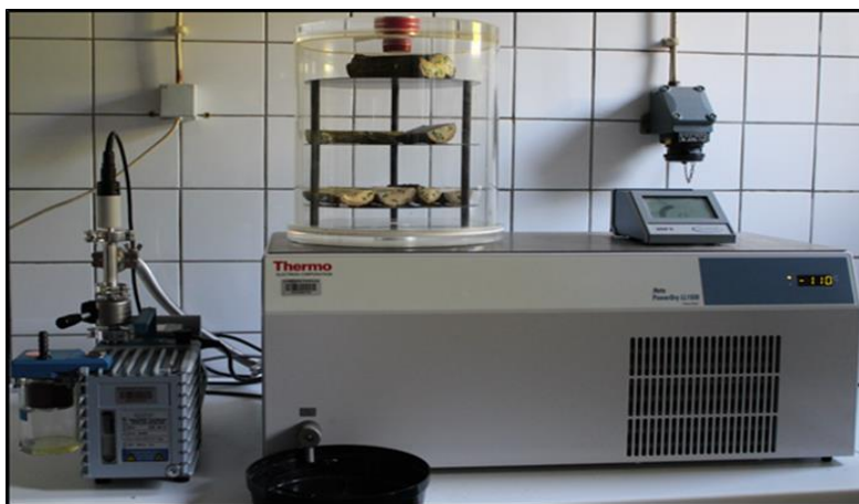
Fig. 4.13: Stem sections containing the wound and inoculation sites are freeze dried.
