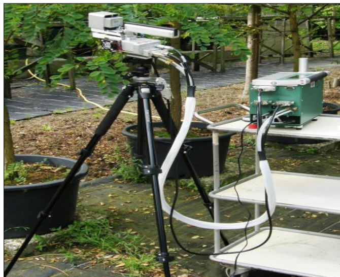
Fig. 4.11: Gas exchange measurements by IRGA; Model LI 6400; LICor Inc., Lincoln, NE, USA.
