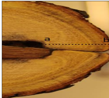
Fig. 4.14. Measuring the callus formation in the vicinity of wounds in all samples of black locust; measurements were taken from a to b.
