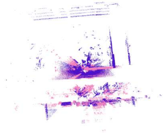
(b) Wrong registration result of 49th and 45th scan pair.
