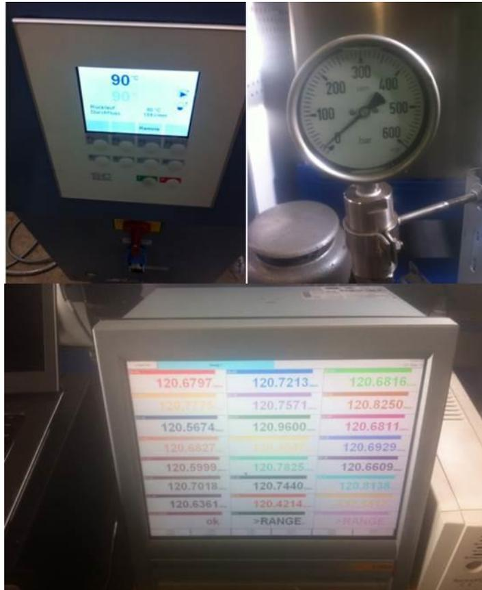
Figure 42 – 42a - Temperature monitoring system at 90°C before the test. Figure 42b - Pressure monitoring system before pressurization of the sample. Figure 42c - Strain gauges reading just after the pressurization of the bore of the sample with supercritical CO<sub>2</sub>.
