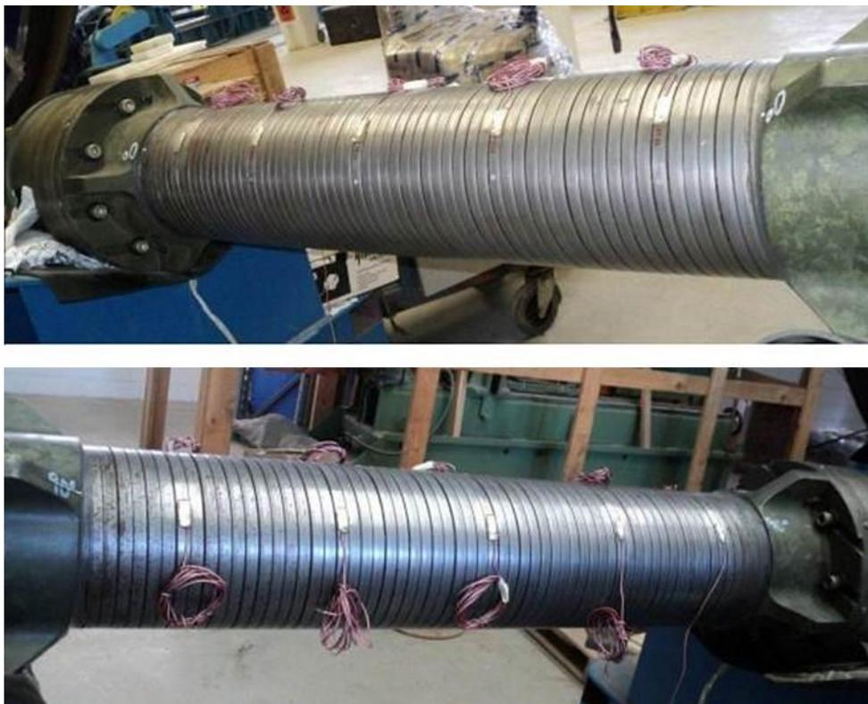
Figure 39 – General view of the sample before the installation of the external steel bars, as well as the insertion of the external shell. General view of some strain gauges along the pipe.
