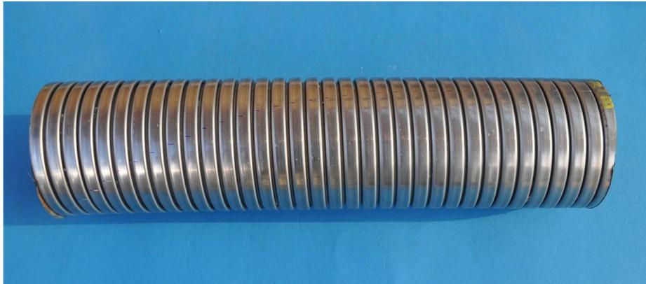
Figure 21 – Carcass subjected to rapid gas decompression test with supercritical CO<sub>2</sub>. No corrosion was verified as this layer is made of stainless steel <sup>(162)</sup>
