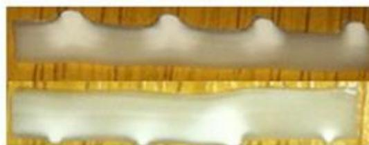
Figure 51 – Correct disposition of each layer in a flexible pipe. Above: Flexwear – 2w and below: Flexbarrier – 2b.
