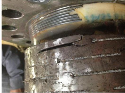
Figure 74 – Broken weld close to one of the sealing regions of the sample, which yielded in the leaking of the CO<sub>2</sub> from the bore of the pipe.
