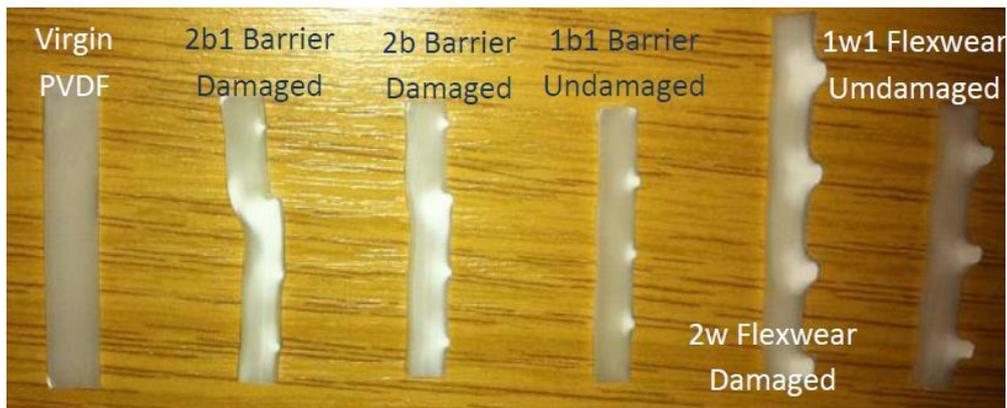
Figure 28 - Virgin PVDF; 2b1 – Flexbarrier sample from damaged region, 2b – Flexbarrier sample from damaged region, 1b1 – Flexbarrier sample from undamaged region, 2w – Flexwear sample from damaged region and 1w1 - Flexwear sample from undamaged region.
