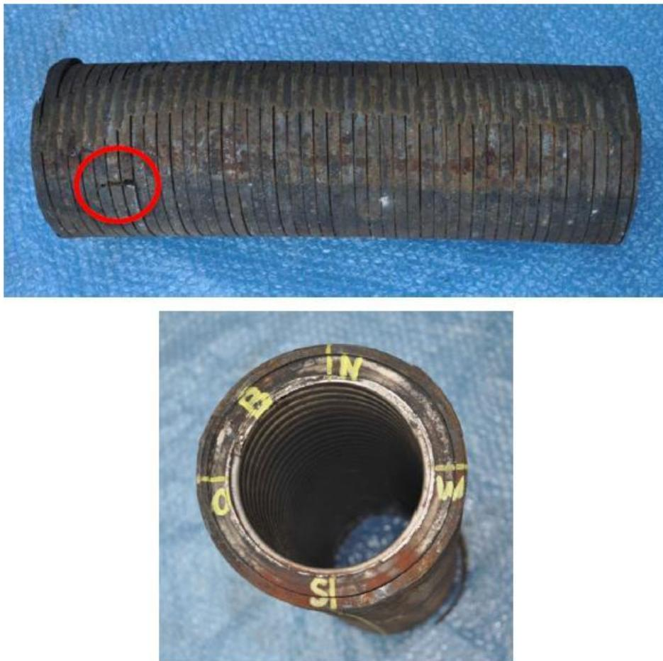
Figure 18 – Segment of a flexible pipe manufactured up to Flexlok, with PVDF Flexwear and Flexbarrier subjected to a Rapid Gas Decompression test with Supercritical CO<sub>2</sub><sup>(162)</sup>
