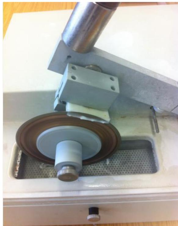
Figure 27 – Slicing process of the PVDF samples with a thickness of 1 mm using Buehler Isomet 4000 low-speed saw.
