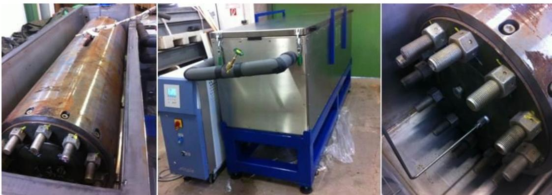
Figure 41 – Figure 41a - Sample inside of tank before being filled with water. Figure 41b - Tank already closed and filled with water just before the test. Figure 41c - Connections used to pressurize the bore of the sample with supercritical CO<sub>2</sub>.
