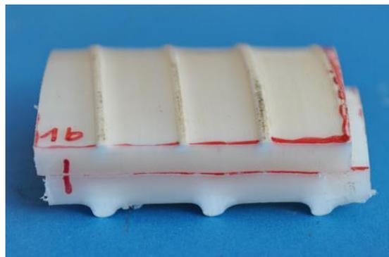
Figure 32 – Specimens 1b and 1w used for SEM investigation from the undamaged region <sup>(162)</sup>
